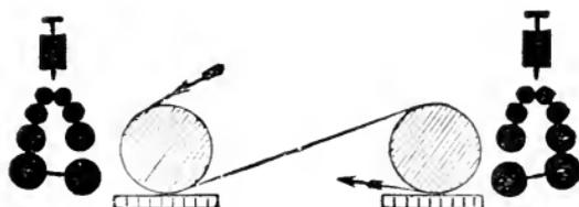
Fig. 4.—Koenig's Double Cylinder for both Sides of Sheet.
