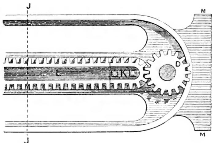
Fig. 28. — Portion of Rack showing position of Teeth and Driving-cog.
