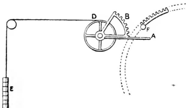
Fig. 9.—“Web” Laying-on Motion—Perfecting Machine.
