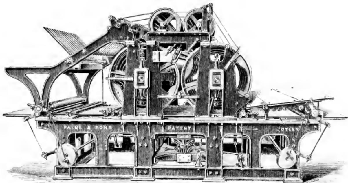
Fig. 37.—Payne's Large Cylinder Single Revolution Perfecting Machine.
