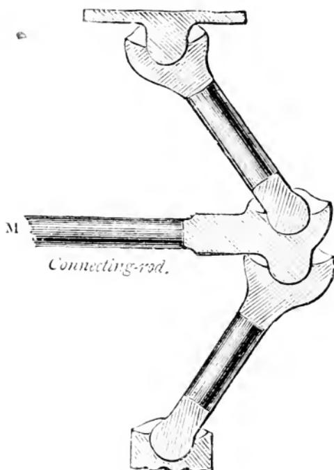
Fig. 25.—Napier's Knuckle Joint.
