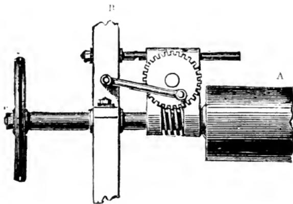
Fig. 11.—A, Ink-drum ; B, Frame of Machine.
