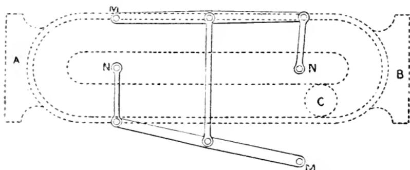
Fig. 29.—Upper side of Rack, showing Parallel Motion.
