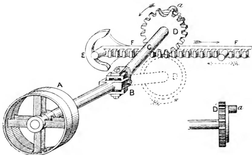
Fig. 35.—Anglo-French Rack and Spindle.
