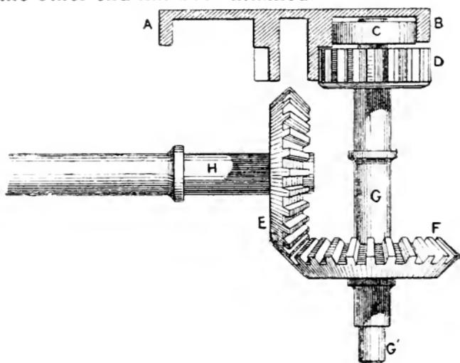
Fig. 27.—Upright Spindle and Section of Rack.
