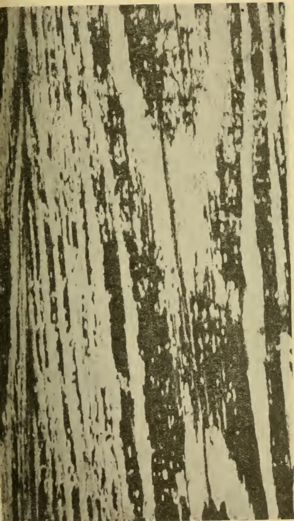
SCALING.—Type of Decay Exhibited by Improperly Made Paint (magnified view).
