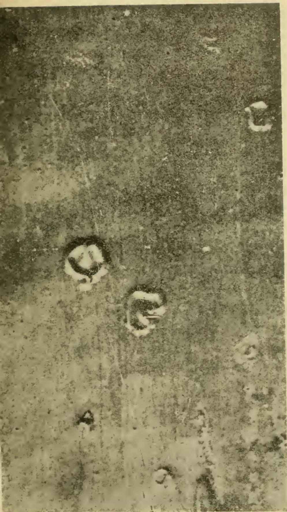
**BLISTERING.**—Type of Decay Exhibited by Improperly Made Paint (magnified view).
