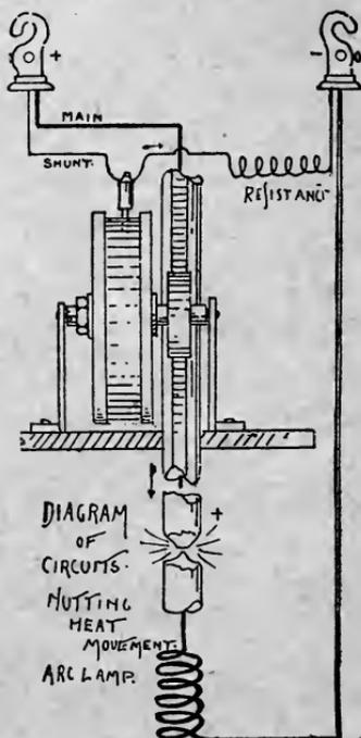
FIGURE 32.—DIAGRAM OF CIRCUITS OF HEAT MOVEMENT LAMP.
