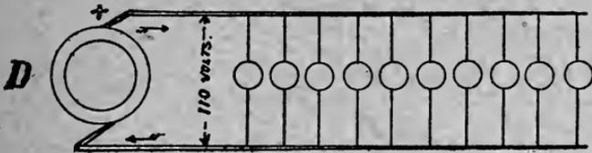
□ FIGURE 20.—SIMPLE MULTIPLE SYSTEM, DYNAMO SUPPLYING 10 LAMPS.
