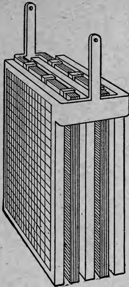
FIGURE 37.—STORAGE BATTERY PLATES.
