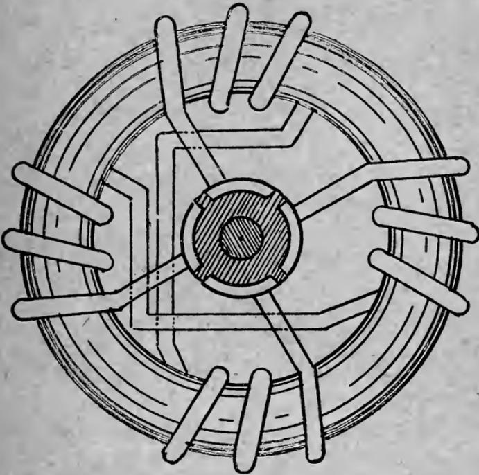
FIGURE 14.—OPEN COIL, RING ARMATURE.
