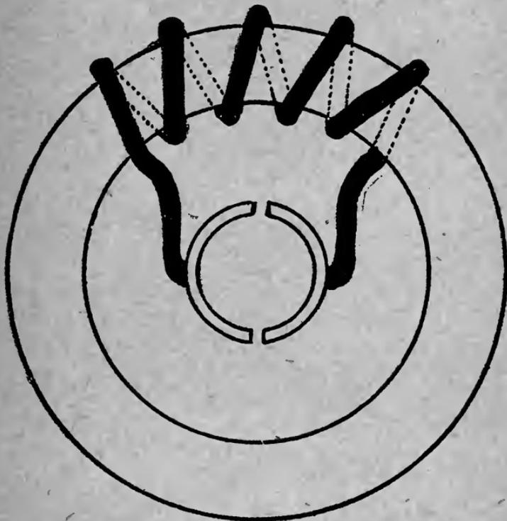
FIGURE 10.—RING ARMATURE OF ONE COIL.
