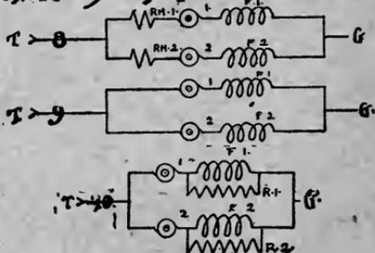
FIGURE 36.—SERIES MULTIPLE STREET CAR MOTOR CONNECTIONS.
