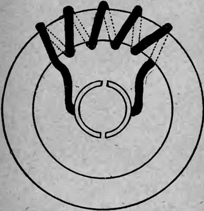
FIGURE 10.—RING ARMATURE OF ONE COIL.
