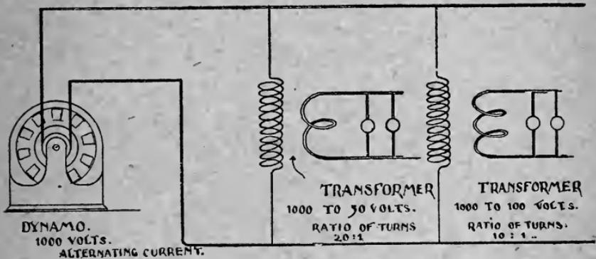
FIGURE 26.—PLAN OF ALTERNATING CURRENT DISTRIBUTION.
