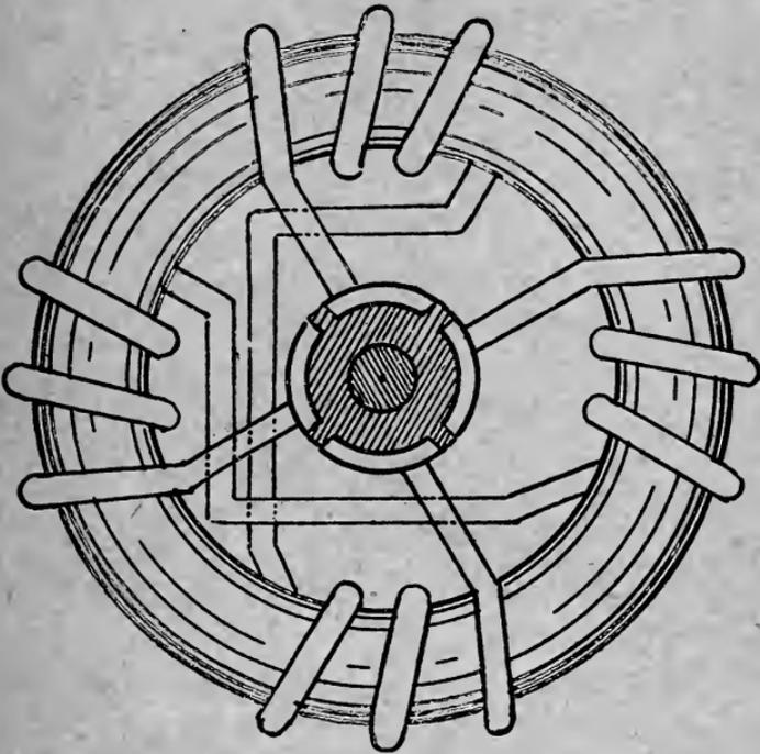
FIGURE 14.—OPEN COIL, RING ARMATURE.
