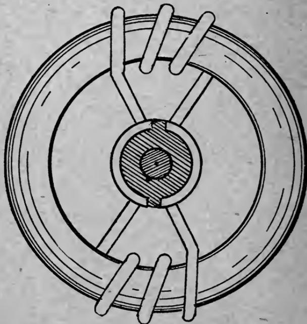
FIGURE II.—RING ARMATURE.—TWO COILS
