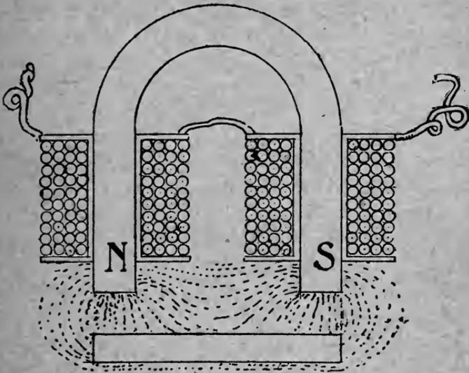
FIGURE 3.—ELECTRO-MAGNET AND ARMATURE SHOWING LINES OF MAGNETISM.
