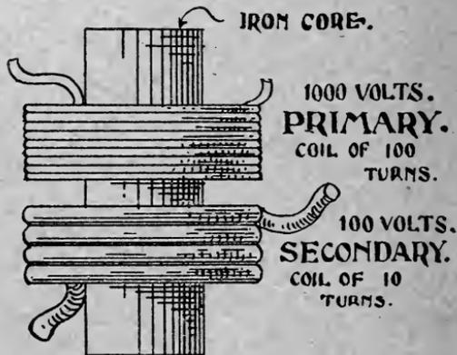
FIGURE 25.—IRON CORE WITH PRIMARY AND SECONDARY COILS.
