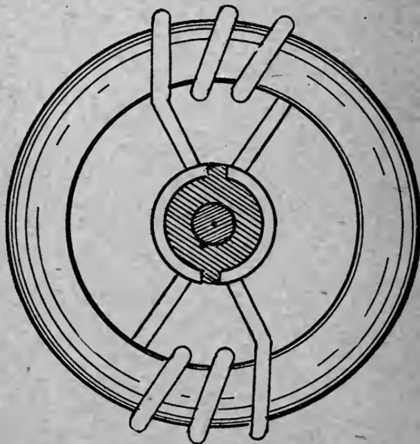
FIGURE II.—RING ARMATURE.—TWO COILS
