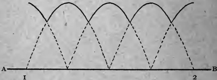
FIGURE 13.—CURRENT WAVES OF FOUR COIL,
