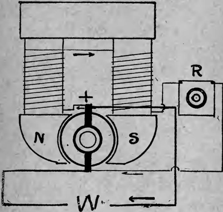
FIGURE 17.—SHUNT WOUND DYNAMO.
