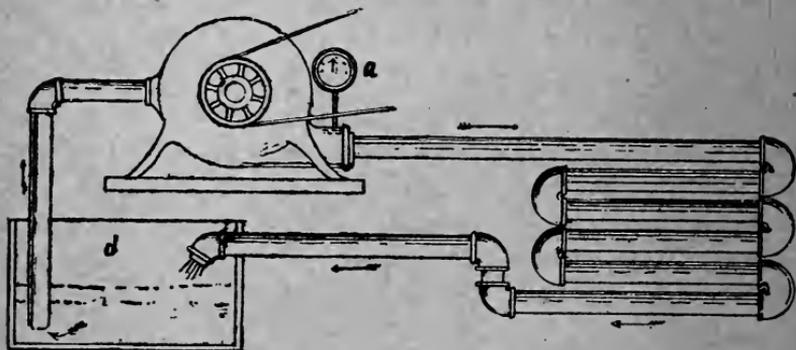
FIGURE 1.—PUMP FORCING WATER THROUGH PIPES.
