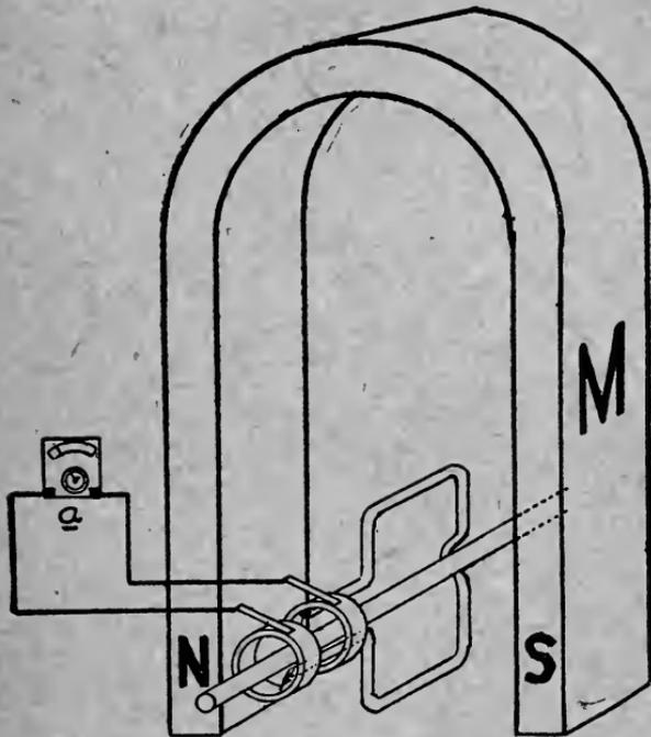
FIGURE 4.—SINGLE LOOP ARMATURE WITH COLLECTOR RINGS, REVOLVING BETWEEN POLES OF PERMANENT MAGNET.
