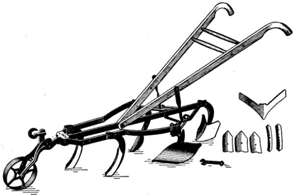
FIG. 5.—A cultivator with wing or hilling teeth.
