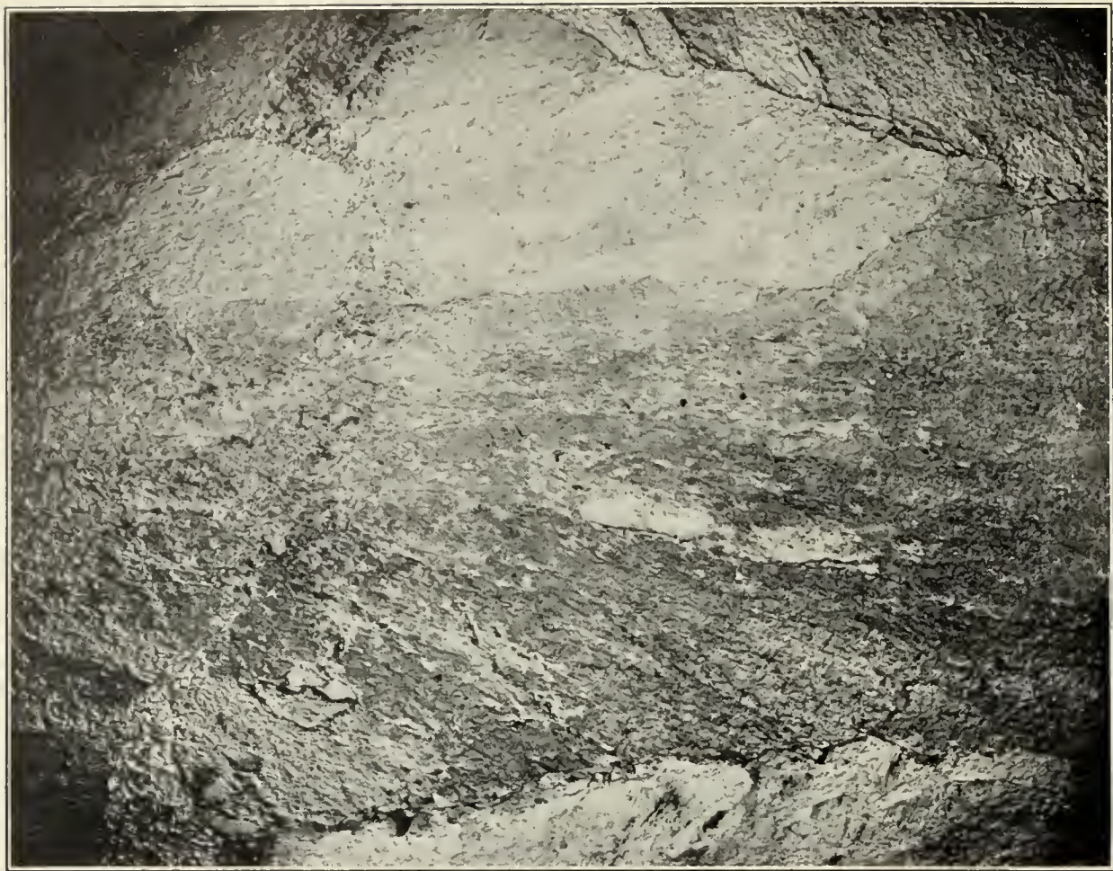
A. PHOTOMICROGRAPH OF SPECIMEN OF ALUNITE FROM TUSHAR RANGE, SHOWING PLUMOSE CHARACTER OF CRYSTALS.
