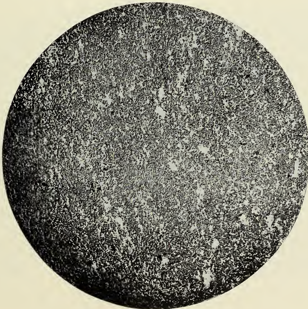
B. PHOTOMICROGRAPH OF SPECIMEN OF HIGHLY ALTERED WALL ROCK ADJACENT TO VEINS FROM GOLD SPRINGS DISTRICT.
