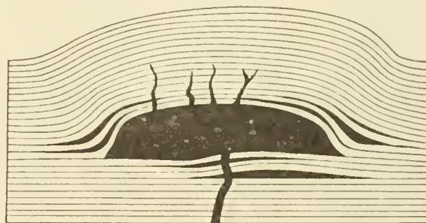
FIGURE 72.—Ideal cross section of a laccolith, with accompanying sheets and dikes. After Gilbert.
