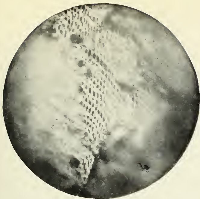
A. PHOTOMICROGRAPH OF CARBONIZED VEGETABLE MATERIAL FROM THE DOLLY VARDEN MINE, SHOWING CELLULAR STRUCTURE.
