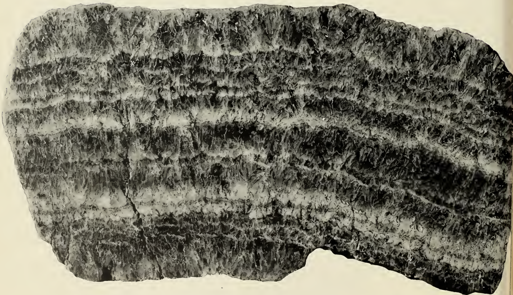
B. SPECIMEN OF ALUNITE FROM TUSHAR RANGE, SHOWING BANDED STRUCTURE OF VEINS.
