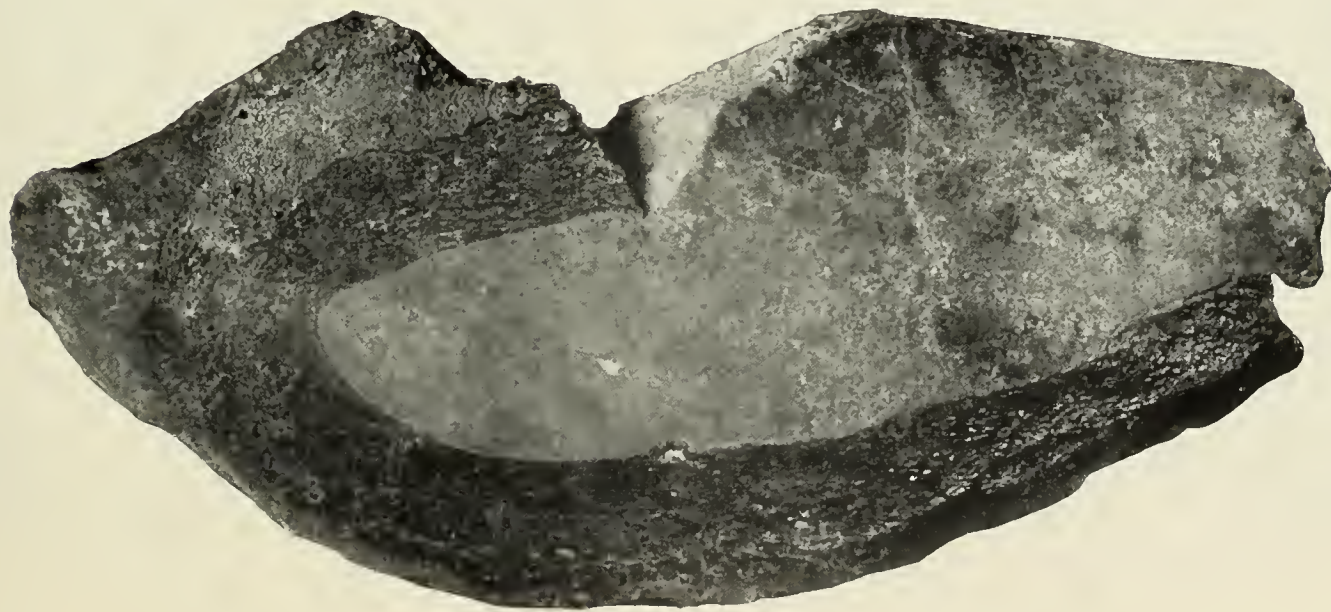
C. COVELLITE REPLACING ZINC SULPHIDE.
