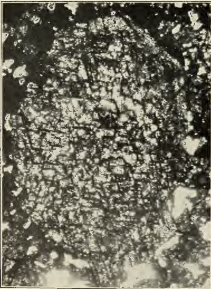
C. PHOTOMICROGRAPH OF CRYSTAL OF ZINC SULPHIDE IN ORDINARY LIGHT.
