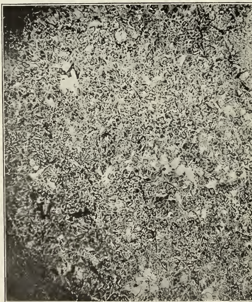
C. PHOTOMICROGRAPH OF SPECIMEN OF VEIN MATERIAL FROM GOLD SPRINGS DISTRICT, SHOWING QUARTZ AND ADULARIA.
