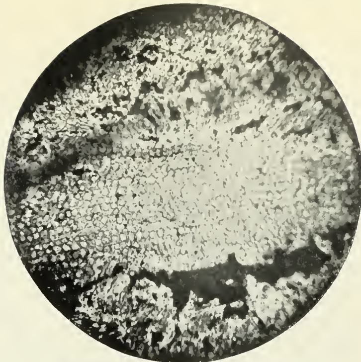
B. PHOTOMICROGRAPH OF VEGETABLE MATERIAL REPLACED BY SULPHIDE FROM THE BLUE DIKE MINE, SHOWING CELLULAR STRUCTURE.
