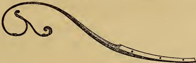
of carriages, which makes a very nice thing. The scroll ends, as seen in the drawing, are filed to the shape of a raised and hollow moulding, or in the form of a thread to a screw.
