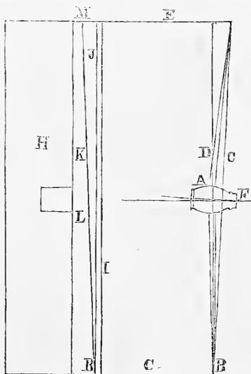
base line C, and each wheel in range with the other also, at point F. By squaring from line G and D, we have the proper set of the axle arm, with a parallel spoke on the under side of the wheel.
