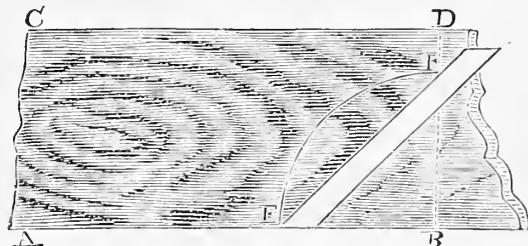
By the help of a mitre square, and a pair of compasses, to square the end of a plank:—Let A, B, C, D be a board of which we wish to make the end square at D, B. Having made the edge A B perfectly straight, assume any point (B, for instance) from which we are required to cut the end square, open the compasses any
