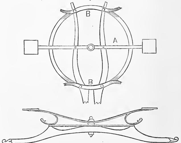
In each diagram A shows the transom stay—the first a bird's eye, and the second a vertical view—which can be raised or lowered to suit the height of the front of the body. In using this stay in place of wood, no furchells are required, the front and back stays being bolted on the fifth-wheel, as shown at B B.
