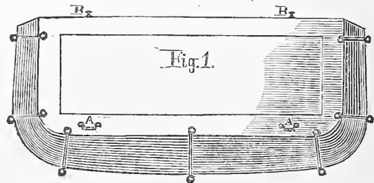
A A in Fig. 1 represent two one-inch check-loops sewed to the seat bottom, two inches from the back side and six and a half from the ends. B B represents two knobs, driven into the front of the seat, as in this instance, or may if chosen, be driven on top, hidden by the cushion. C C (Fig. 2) are two hard pieces of leather stitched upon
