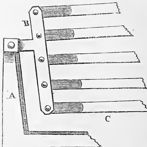
hinged to the T by rivets, as before stated, to take the bows. For carriages—such as landaus—this arrangement of the bows is a decided improvement over the old one, especially when applied to the front half of the head, as, in falling, the lower bows are thrown back, thus clearing the dickey-seat and allowing of a shorter coupling. This, we believe, is public property and unpatented.
