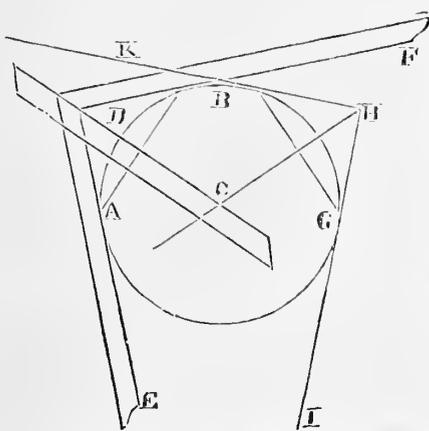
Let A B G, be any circle or part of a circle to which apply your square so that the inside edge of the blade and stock shall touch it as at A and B, shown in the figure; then take your miter-square and place it at the angle D of your square, and draw a line along its edge, as
