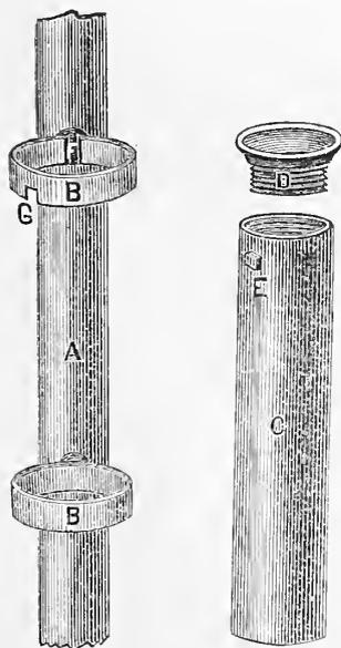
The invention of Mr. Fourier consists: 1st. In the use of metal rings made stationary, either on the railing of the dash, or on an iron stay made expressly for it at any desirable place. 2d. In having the socket in two pieces; which makes it more solid, and allows of taking off. In this way the whip has firm hold, and can neither swing to the right nor left, taking the badly-affixed socket with it.
