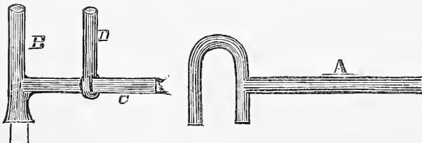
A shows the hand bending lever. The upright in B is forged solid with the arm C, at right angle. This arm C should be swaged oval, for the purpose of keeping the sliding iron D in its place, whenever it is set for either a larger or smaller iron, or for long or short sweeps. If
