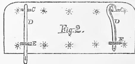
the inside, with the ends of the straps, D D, upon the outside of the cushion bottom. E E show two hard leather checks, stitched fast upon the outside of the cushion, through a piece of leather on the inside.
