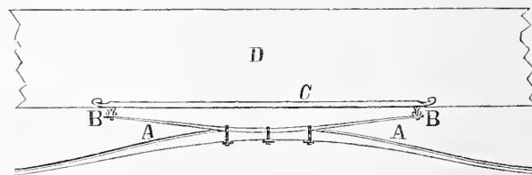
In the diagram, AA is a single-leaf spring, nicely bedded on the top of the side-bar, and secured thereto by three light clips, the side-bar itself resting on half springs at the ends. BB are the ends of two cross-bars on which the body D rests; and C a light wooden bar connecting with the ends of bars BB, through which it is bolted to the ends of the spring.
