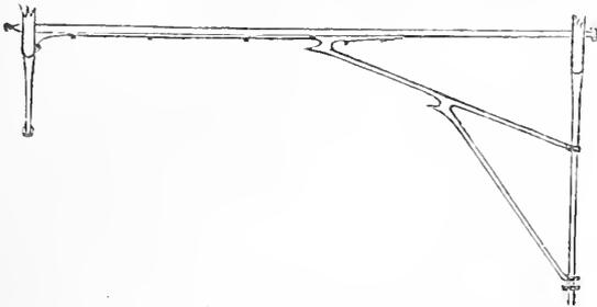
the same manner as those used for coaches, the side-plates running back of the point where the stay strikes the perch in order to strengthen it. For a light buggy these stays are made of  $\frac{3}{8}$  or  $\frac{7}{16}$  round iron. These look much lighter and are stronger than oval.
