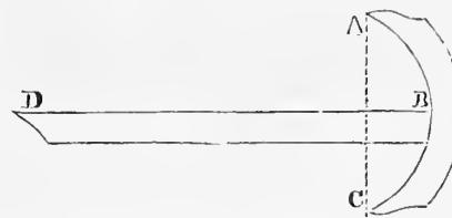
A and C should have a small piece of hardened steel affixed, so that it should not be subject to wear by use, into which stock, the blade
