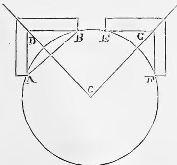
Now in order to show how this is done, let A B E F be the circle, and A D B the square. Having the blade A D equal in length to the stock B D, apply it, as shown in the figure, so that the ends meet the circle at the points A and B, and with a miter-square draw a line in the direction D C, which will tend to
