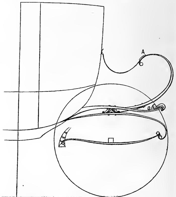
back is bound with an iron finishing in a scroll on the top end of the spring like the drawing at A. From this point an iron stay extends to and is attached to the body. The iron is afterwards covered with patent leather, so as to give it the imitation of a check-strap in the real form. When nicely finished, the job has a very pleasing effect and to the superficial observer looks like the real article.
