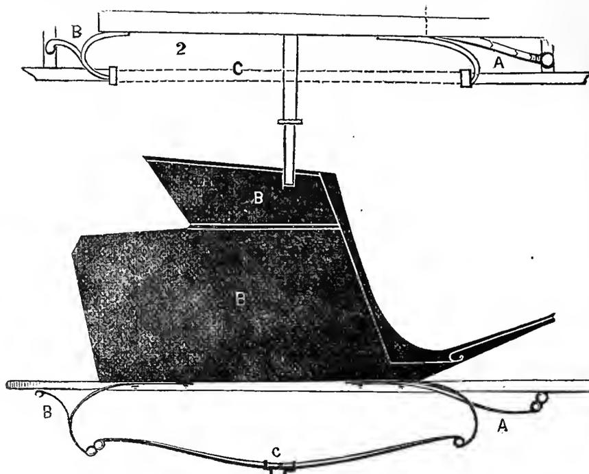
is received in a knuckle on the back shaft bar of such peculiar form as to permit the shafts to play up and down without straining the irons.
