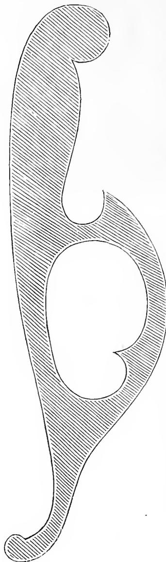
taken to file the edges of the sweeps true, and a little rounding, so as to make it work well afterwards when running your pen or pencil along the edges.
