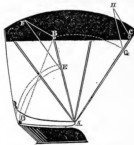
diagram,) where the third bow will come when down even with the top props D, by taking a thread and hanging it on point A; next draw with the thread and a piece of chalk the circular line—in dots—from D to the third bow at E, and mark it; then hang the same thread on prop B, measuring to prop D; then move with that length from D to joint E, doubling the cord to suit as you see it marked on point F. In that position will the top joint stand when the top is down.
