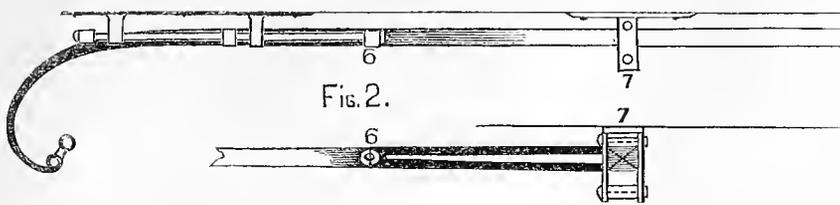
shafts, at the hind end, from the knuckle-joints 6, 6, is iron, the projections for the slide-bolts being welded on solid.
