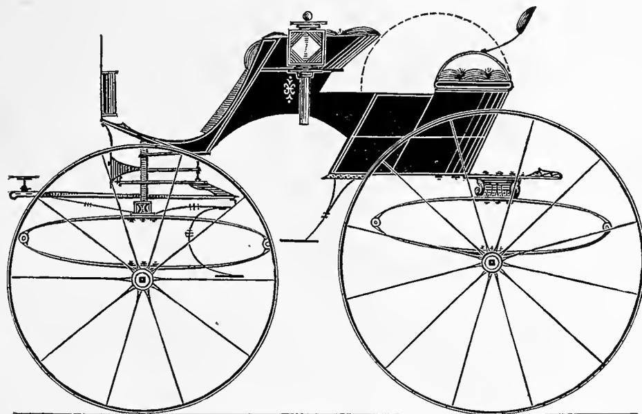
PHAETON, WITH SEAT TO TURN IN.— $\frac{1}{2}$  IN. SCALE.
