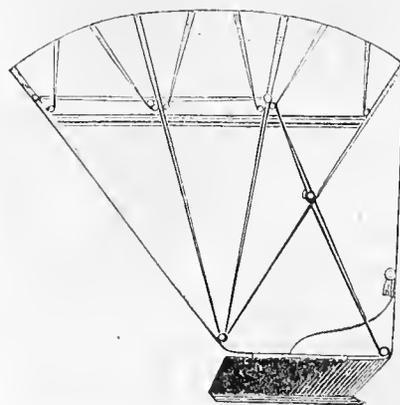
ment here illustrated will most effectually prevent it, and preserve the head in its original beauty, as will be seen from the diagram. This is accomplished by fixing smaller and shorter bows between the longer ones, on a pivot, so as to fall almost as flat when down, as in the common method. Shop or county rights to use this improvement can be had
