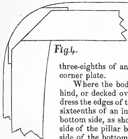
corner with the inside lightened out, having been done beforehand in the vise, with knife and plane, and you have only to bring the top edge to about three-eighths of an inch, and screw on a corner plate.
