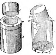
Fig. 4 - Varnish Brush Keeper.
