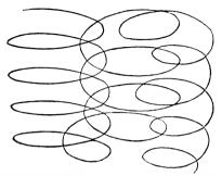
Fig. 19—The Motions in French Polishing.
