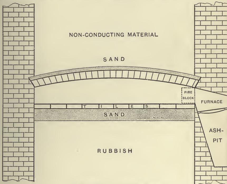
Fig. 199.—Section of Oven through Furnace
