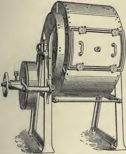
Fig. 220.—Hawkins Rotary Dough-making Machine
