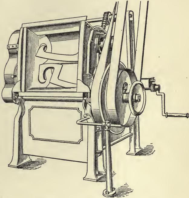
Fig. 218.—"Universal" Kneading Machine, Tilted
