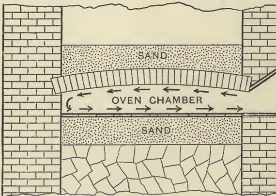
Fig. 198.—Section of Side-flue Oven
