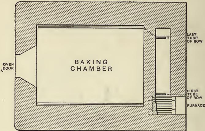
Fig. 211.—Hawkins' Patent Regulated Steam-pipe Oven: Plan
