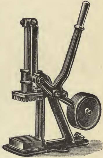
Fig. 142.—Chip-potato Machine
