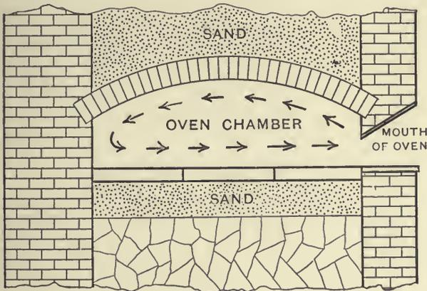
Fig. 195.—Section of Modern Scotch Oven
