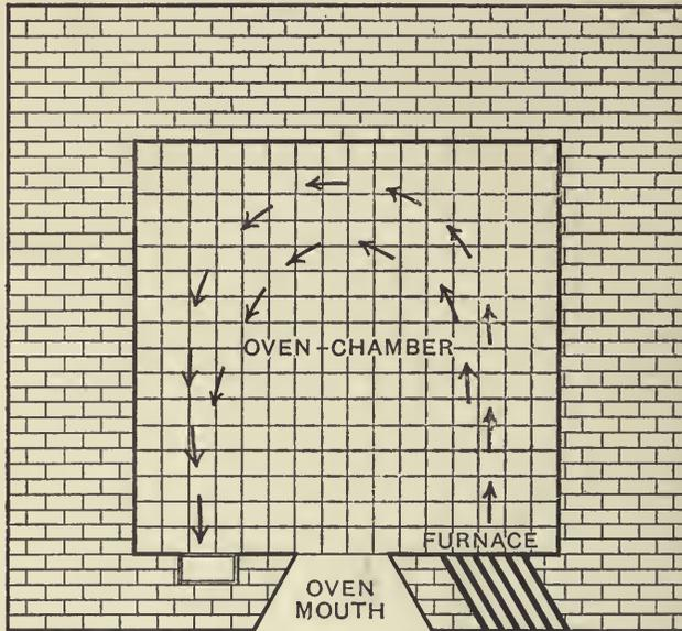
Fig. 197.—Plan of Side-flue Oven
