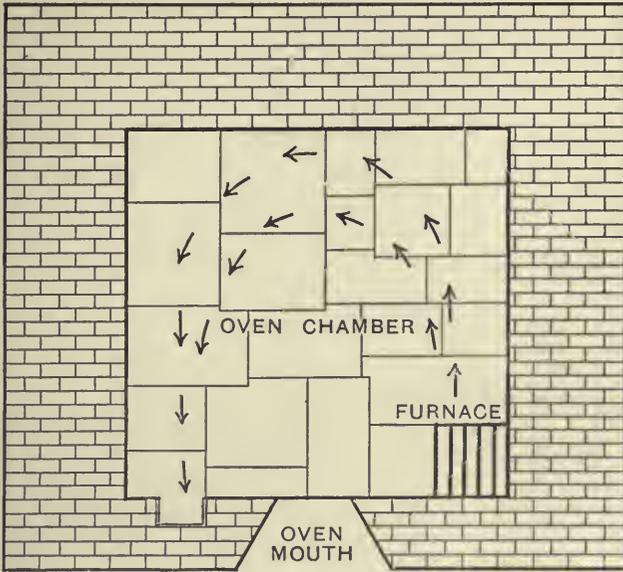
Fig. 194.—Plan of Modern Scotch Oven
