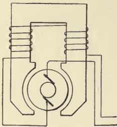
Fig. 225.—Diagram of Series Winding
