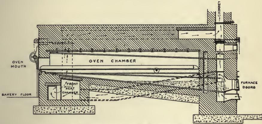
Fig 209.—Baker's Patent Steam-pipe Drawplate Oven
