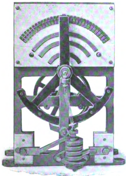
FIG. 505.—AUTOMATIC REGULATOR TO CONTROL SPEED OF FLYWHEEL.
