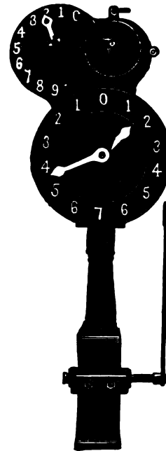
FIG. 632. SIGNAL BELL AND WINDING INDICATOR.
