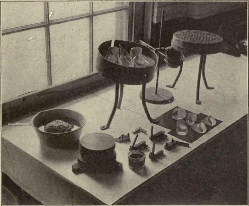
FIG. 79.—Prisms in process of blocking with plaster of paris for polishing. On the right there is a block of prisms ready for polishing. (Frankford Arsenal.)
