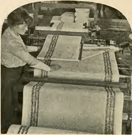
DOUBLING AND WINDING
