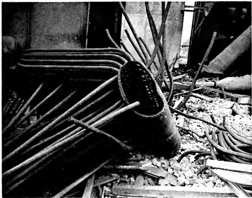
Figure 2—Weakened by corrosion, the blind head in the mud drum of this water tube boiler in a utility plant tore loose and caused the death of four people, injuries to six others and $100,000 property loss.
