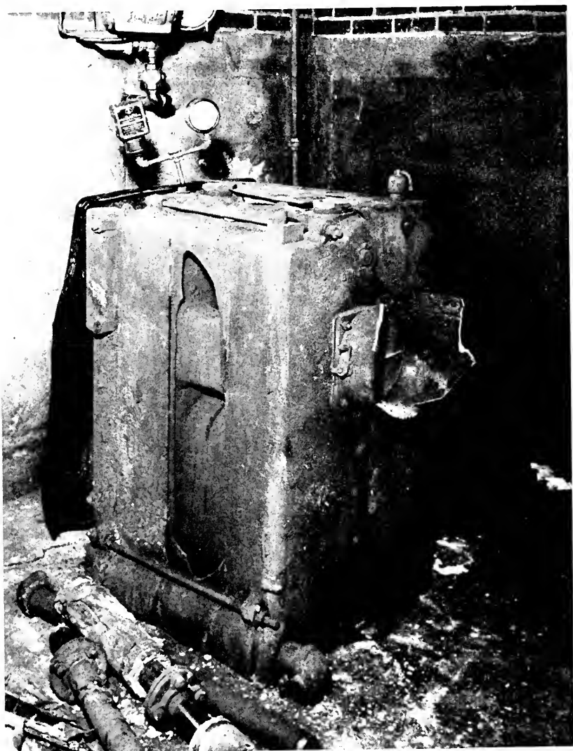
Figure 4—Failure of a pressure control device plus an inoperative safety valve caused the explosion of this cast iron steam heating boiler in a Kansas residence.
