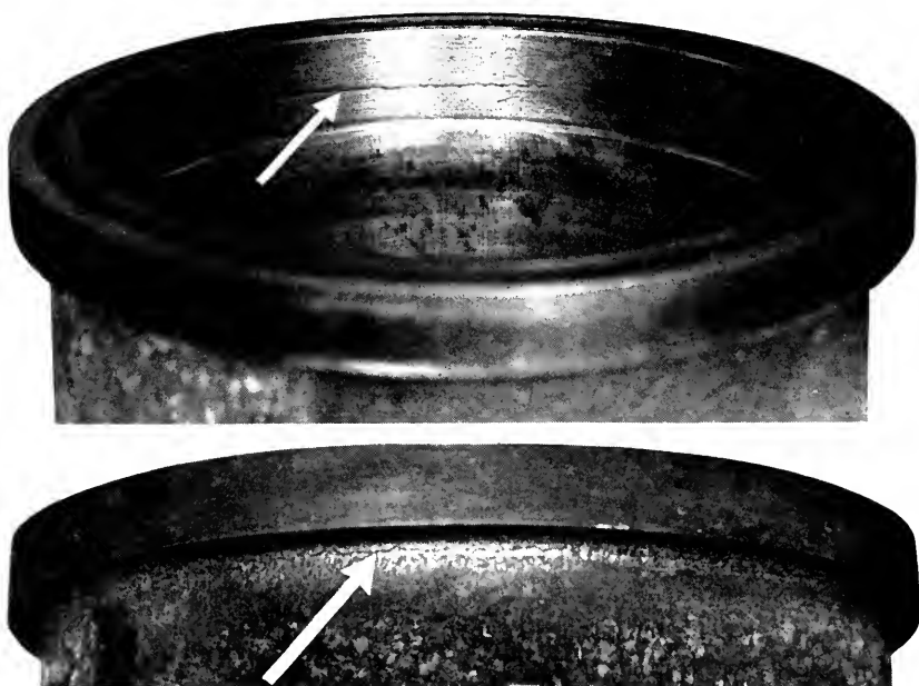
Figure 2 and 2A—Views showing a circumferential crack near the top of a 15" cylinder liner. This crack permitted leakage of water into the cylinder.
