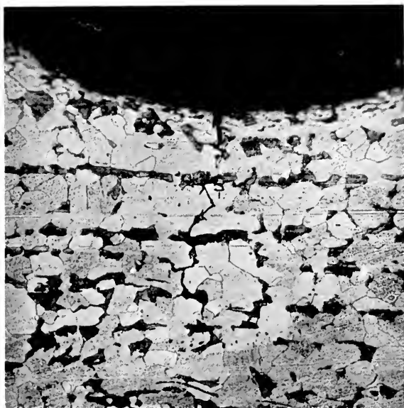
Figure 2—Embrittlement at 225 magnifications. The defect shown here was produced in the University of Illinois tests. The progress of the fissure may be compared to that in Fig. 3.
