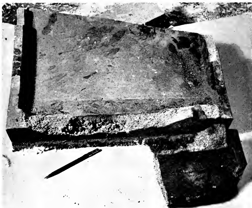
These two broken parts of the wheel, placed together as they were located in the rim, show slag and gas pockets in the casting.
