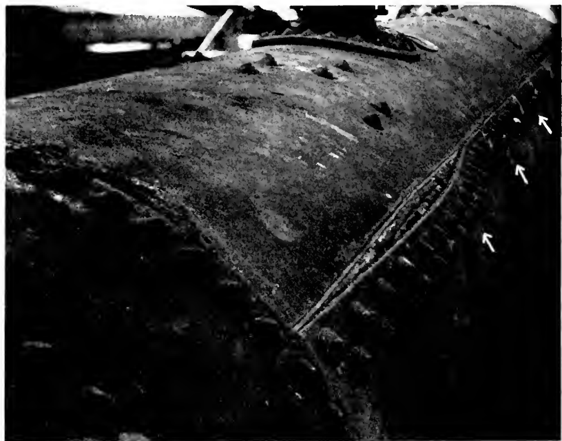
Figure 3—Failure in the longitudinal seam of No. 1 boiler during the hydrostatic test. A few of the paths of embrittlement defects are exposed and clearly show the progress from rivet hole to rivet hole. This boiler has been slotted as a means of detecting a lap seam crack. The slots are indicated by the arrows. See also Figure 4.
