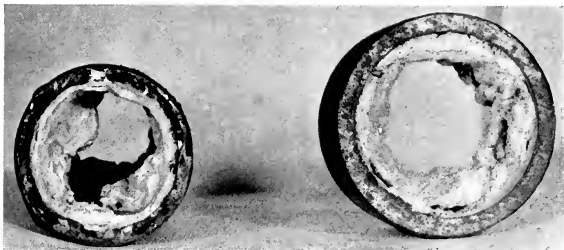
Figure 2—Superheater tubes from two boilers in widely separated parts of the country. Carry-over of solids in the steam rapidly builds up such deposits.
