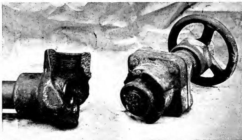
Figure 2—View of the broken by-pass valve which led to the violent explosion described on Page 203.
