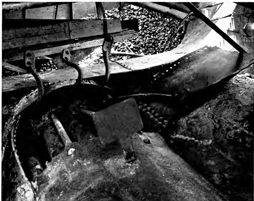
Figure 1—The failure in Boiler No. 2. The break along the rivet holes near the caulking edge of the seam at the left is clearly evident.
