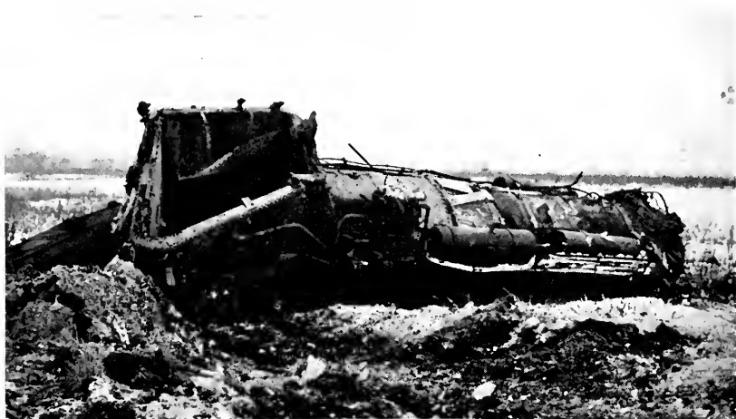
Figure 3—Weighing more than 40 tons, this track locomotive boiler was hurled 500' when low water caused failure of the crown sheet.
