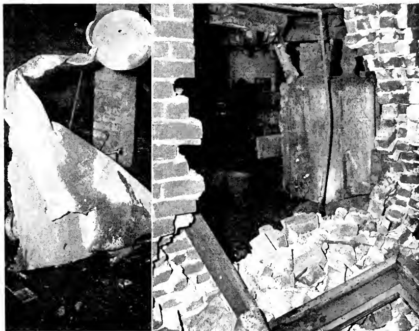
Figure 5—Left—Hot water tank after its explosion. Right—Hole in brick wall made by the exploding tank.
