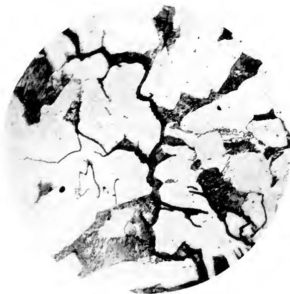
Figure 3—Embrittlement at 500 magnifications. This defect developed in a boiler under ordinary operating conditions. The characteristic intercrystalline path of the disintegration is clearly shown and is directly similar to the disintegration produced in the laboratory and shown in Figure 2.
