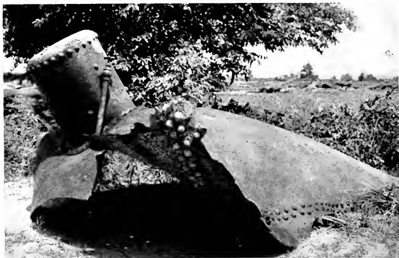
Figure 1—A crack in a longitudinal lap-seam caused the explosion of this boiler. Three men were killed and twelve others injured, eight of them seriously.
