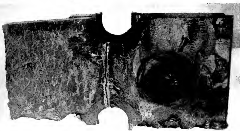
Figure 2—A fully developed embrittlement defect in metal from one of the steamer's boilers. The lower picture shows the rivet hole to rivet hole direction of the disintegration. The top picture is of the same pieces of metal as the lower, the dark areas in the break illustrating the development of the embrittlement (see arrows).
