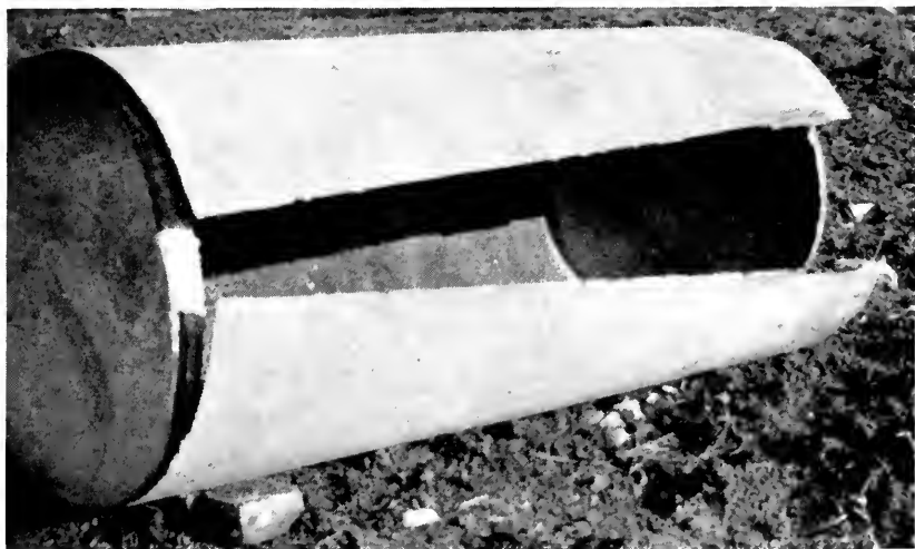
Figure 3—Failure of the longitudinal seam. Faulty welding was given as the cause of this accident.
