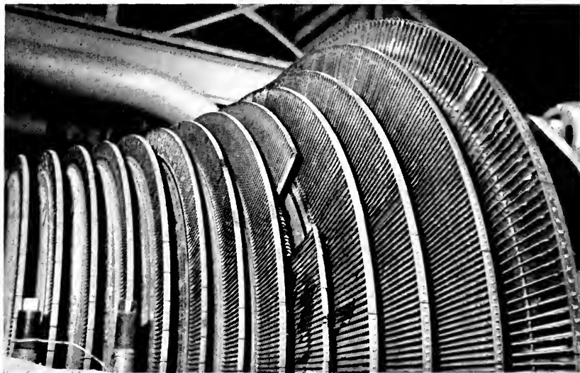
Figure 1—Part of the upper half of a 23,000 kw steam turbine showing damage to the nineteenth stage wheel when a 12" section of the disc broke near the rim. The cause was attributed to a progressive crack.
