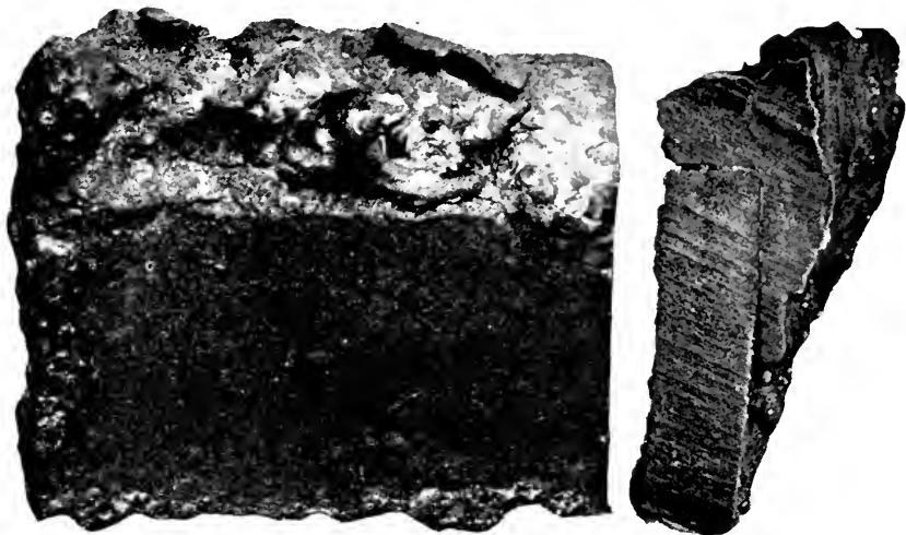
Figure 1. An example of uncontrolled welding. Parts of a 36" x 24" patch on a high pressure boiler are shown. The patch was welded flush with the shell plate and there was very little fusion. How little may easily be ascertained from the photograph at the right showing the cross section of the seam.
