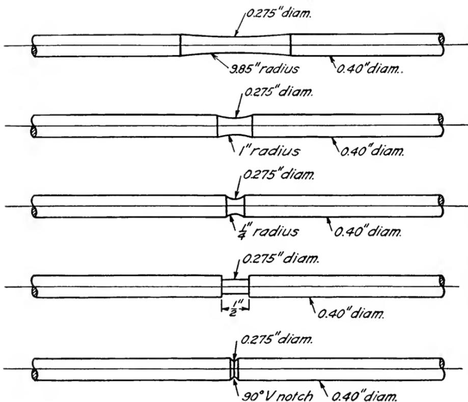
FIG. 4. SHAPES OF SPECIMENS TESTED.
