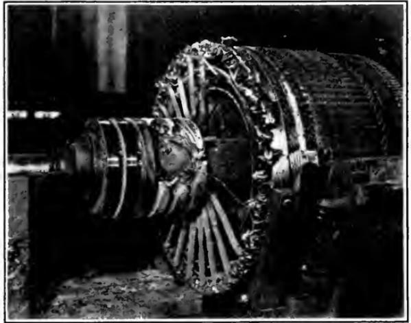
ARMATURE BURNOUT OF ROTARY
