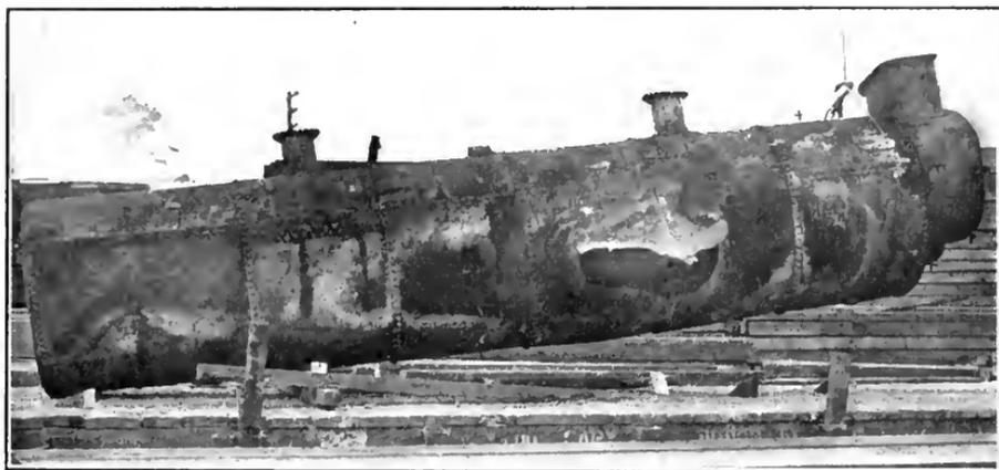
BOILER BURNED AND RUPTURED AS A RESULT OF LOW WATER.
