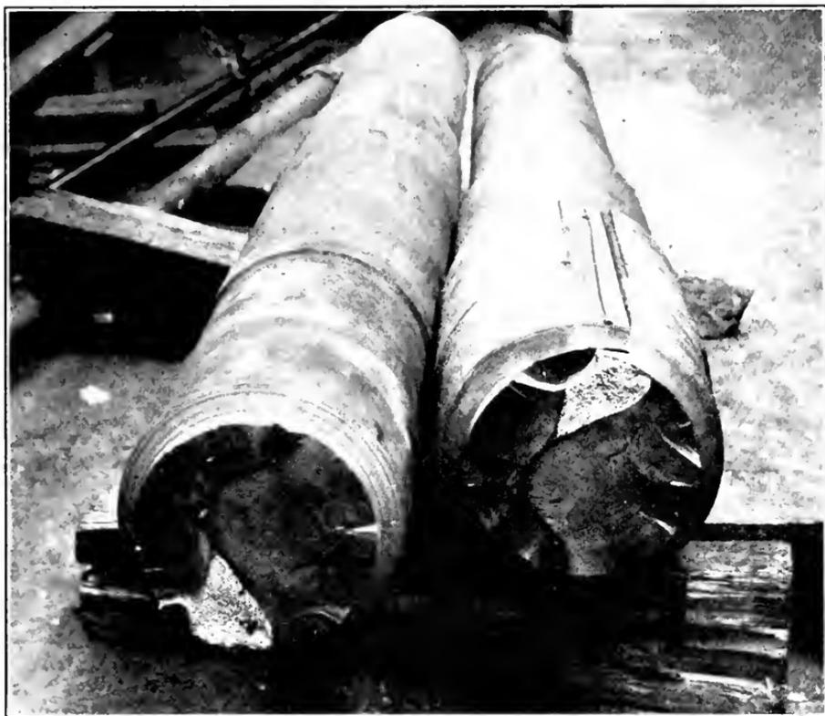
FAILURE OF SHAFT CAUSED BY WELDING.
