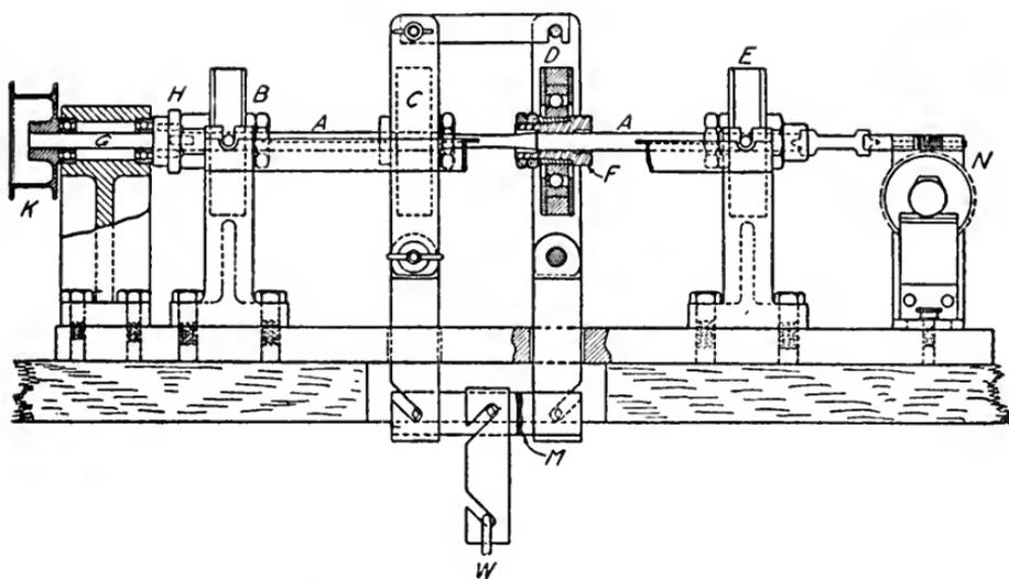
FIG. 1. ROTATING BEAM TESTING MACHINE (FARMER).
