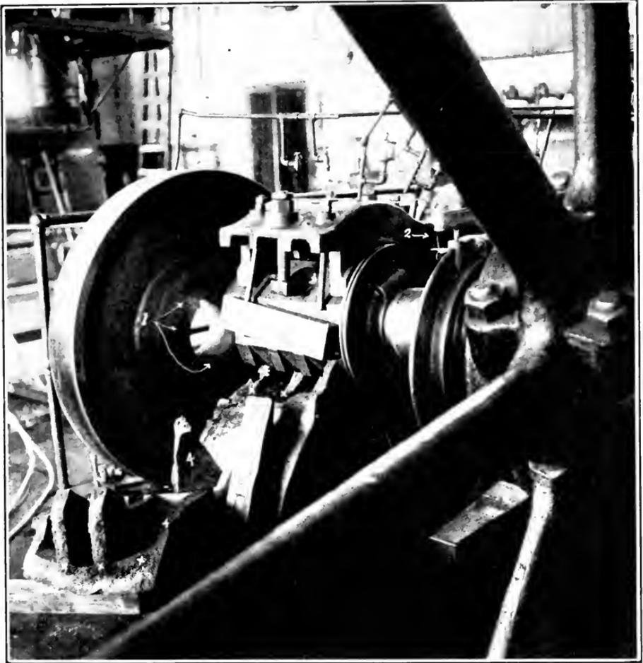
ENGINE WRECKED BY WATER IN CYLINDER.
