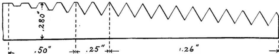
FIG. 5.—SECTION THROUGH A SIX-INCH PIPE.
