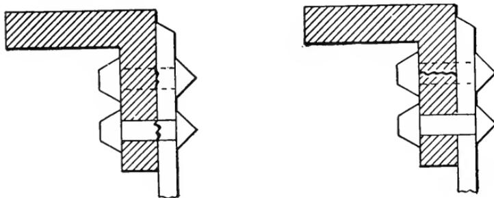
FIGS. 2 AND 3. — METHODS OF FAILURE OF THE RING.
