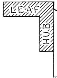
FIG. 7. — NAMES OF THE PARTS OF THE RING.
