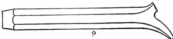
FIG. 9. — BEADING TOOL. (HAND.)
