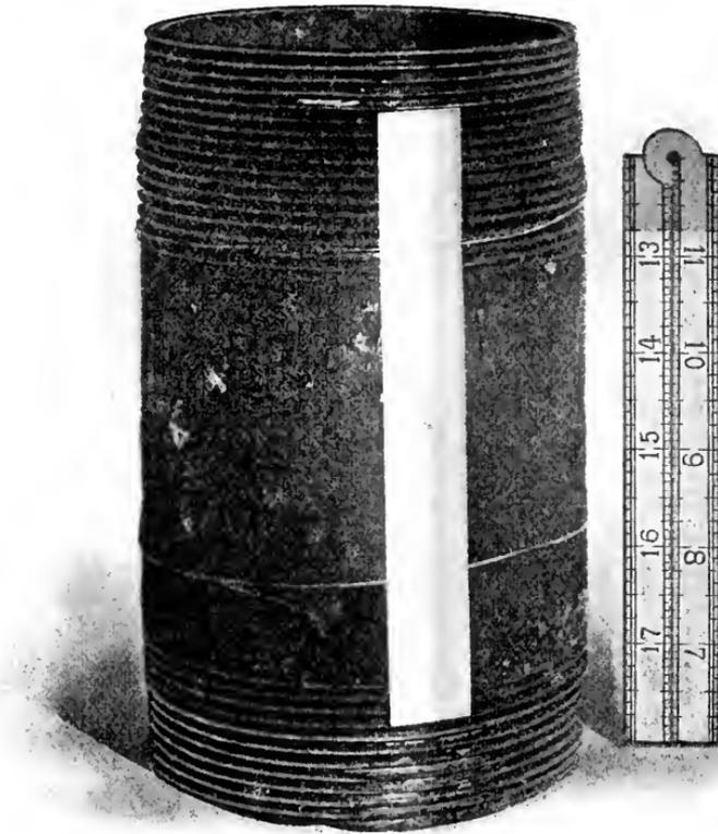
FIG. 7. — FOUR-INCH PIPE. THREAD WITHOUT SUFFICIENT TAPER; MADE UP ONLY FOUR THREADS.
