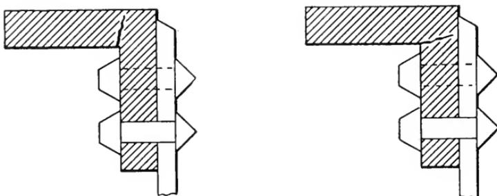
FIGS. 4 AND 5. — METHODS OF FAILURE OF THE RING.
