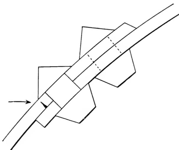
FIG. 11.—ILLUSTRATING THE HIDDEN CRACK WHICH CAUSED THE EXPLOSION.
