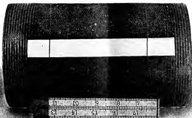
FIG. 8. — FIVE-INCH PIPE; STANDARD (OR NEARLY SO) AT ONE END, BUT NOT AT THE OTHER.
