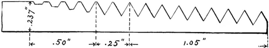
FIG. 3.—SECTION THROUGH A FOUR-INCH PIPE.
