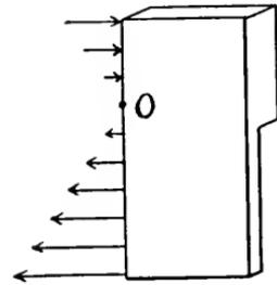
FIG. 26. — ILLUSTRATING THE CIRCUMFERENTIAL TENSIONS.
