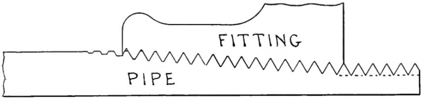
FIG. 13. — ILLUSTRATING THE PIPE PROJECTING THROUGH THE FITTING.
