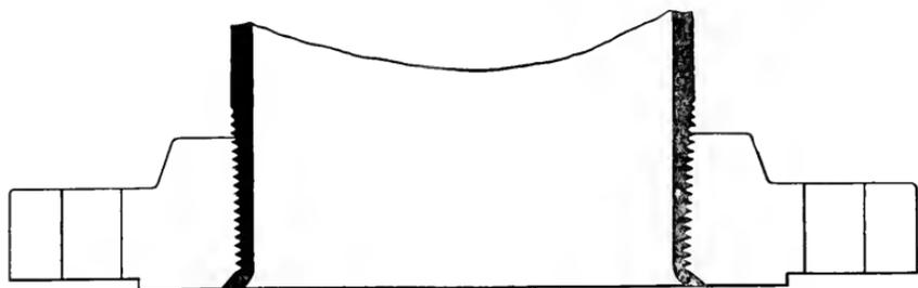
FIG. 10. — ILLUSTRATING A PEENED PIPE.
