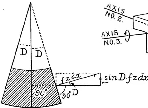
FIG. 29. — RESOLUTION OF THE CIRCUMFERENTIAL TENSION.
