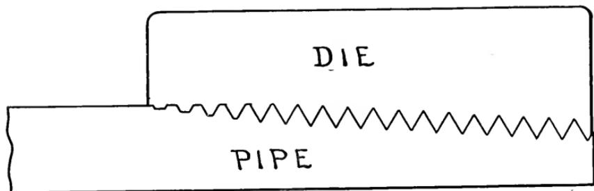
FIG. 11. — ILLUSTRATING A COMPLETED PIPE THREAD.
