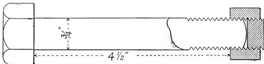
FIG. 1. — SHOWING "STUB END" OF BOLT IN POSITION.
