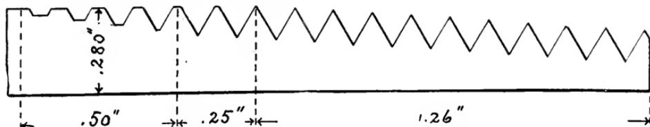
FIG. 5.—SECTION THROUGH A SIX-INCH PIPE.
