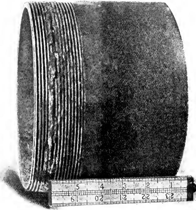
FIG. 9.—EIGHT-INCH PIPE, WHICH COULD BE MADE UP ONLY THREE THREADS.
