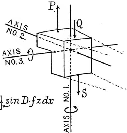
FIG. 30. — THE THREE AXES OF ROTATION.
