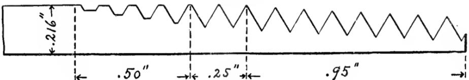
FIG. 2. — SECTION THROUGH A THREE-INCH PIPE.
