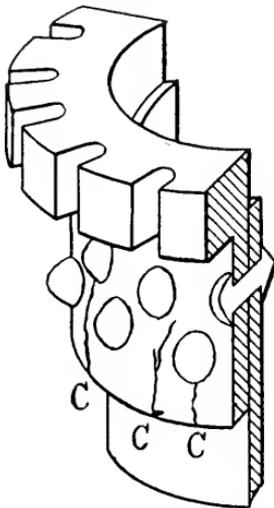
FIG. 6. — SHOWING "HUB CRACKS."
