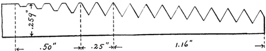
FIG. 4.—SECTION THROUGH A FIVE-INCH PIPE.
