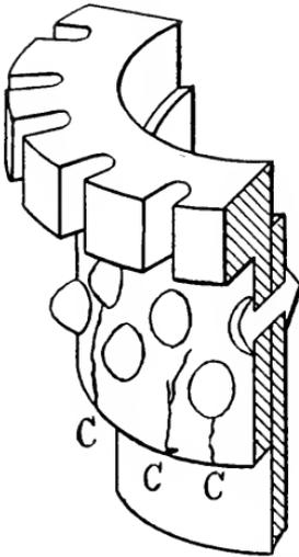
FIG. 6. — SHOWING "HUB CRACKS."
