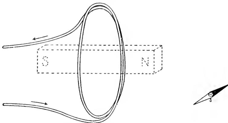
FIG. 1. — ILLUSTRATING THE PRINCIPLE OF THE GALVANOMETER.
