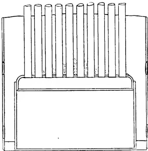
FIG. 2. — LOOSE DEPOSIT ON TUBE SHEET.
