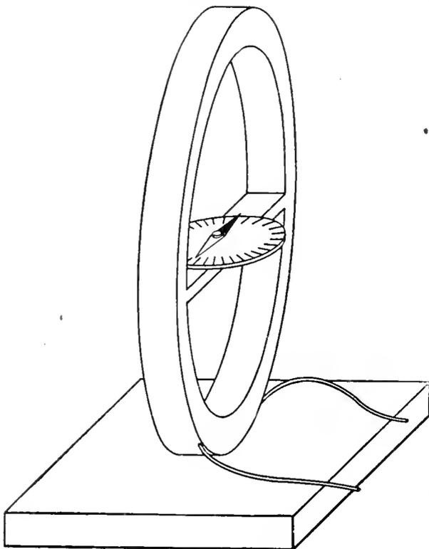
FIG. 2. — A GALVANOMETER.
