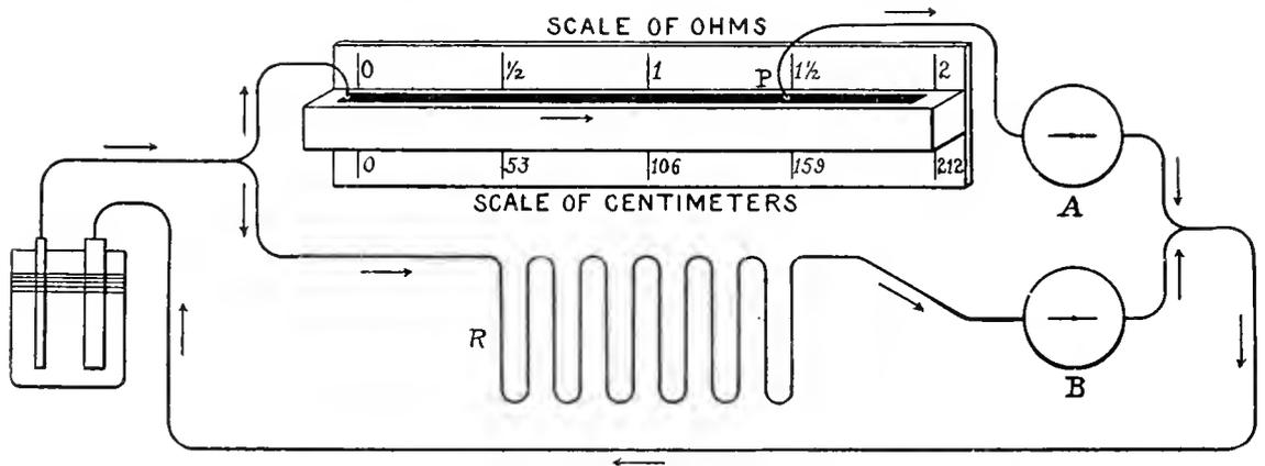
FIG. 7. — ILLUSTRATING THE MEASUREMENT OF RESISTANCE.
