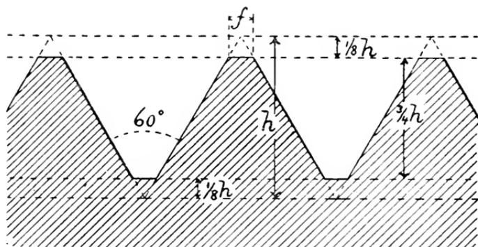
FIG. 1. — DIAGRAM OF THE SELLERS THREAD.
