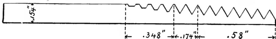
FIG. 1. — SECTION THROUGH A TWO-INCH PIPE.
