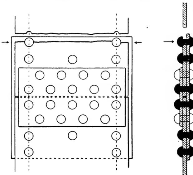
FIG. 2.—FRACTURE THROUGH OUTSIDE ROW OF RIVETS.
