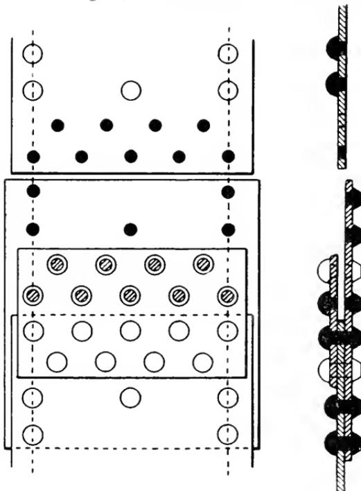
FIG. 6.—ALL THE RIVETS SHEARED.
