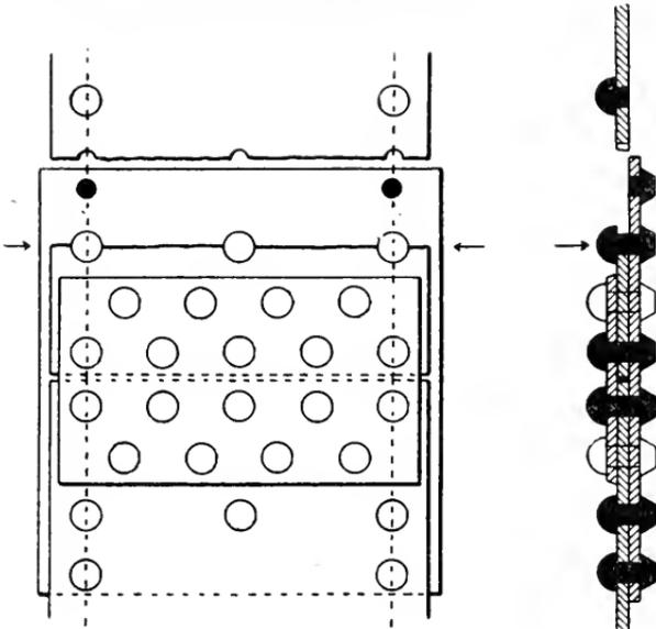
FIG. 3.— FRACTURE THROUGH THE NEXT-TO-OUTSIDE ROW OF RIVETS.
