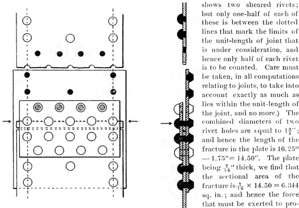
FIG. 5.—FRACTURE THROUGH THE INSIDE ROW OF RIVETS.
