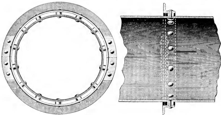
FIGS. 4 and 5.—RING OF ANGLE-IRON, WITH THIMBLES.
