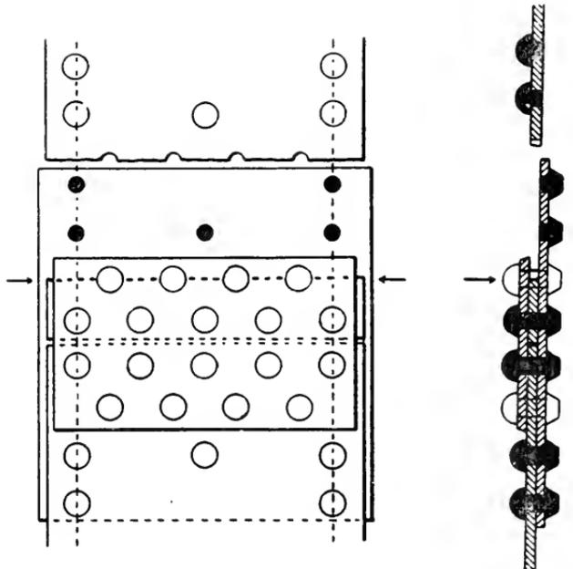
FIG. 4.— FRACTURE THROUGH THE NEXT-TO-INSIDE ROW OF RIVETS.
