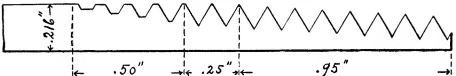
FIG. 2. — SECTION THROUGH A THREE-INCH PIPE.
