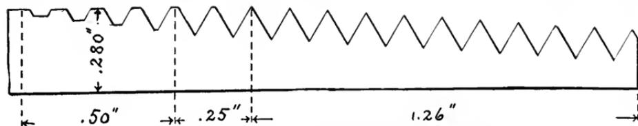
FIG. 5. — SECTION THROUGH A SIX-INCH PIPE.
