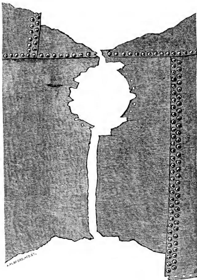
FIG. 2.— THE INITIAL RUPTURE THROUGH THE MAN-HOLE.
