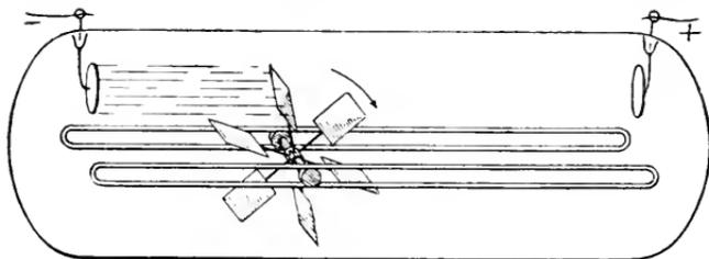
FIG. 3.—CROOKES' "RAILWAY" TUBE.
