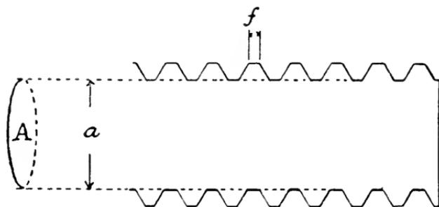
FIG. 2. — ILLUSTRATING "DIAMETER AT ROOT OF THREAD," ETC.
