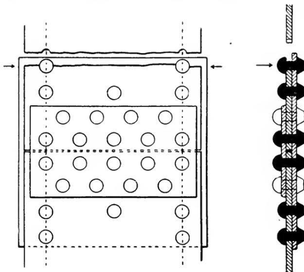
FIG. 2.—FRACTURE THROUGH OUTSIDE ROW OF RIVETS.
