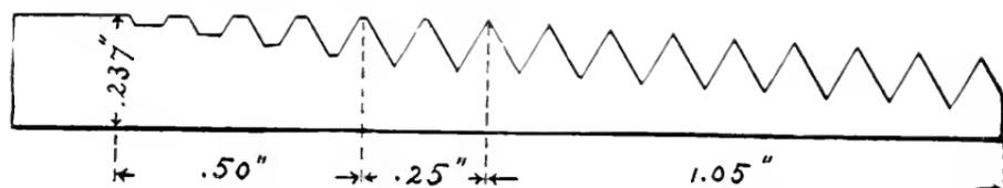
FIG. 3. — SECTION THROUGH A FOUR-INCH PIPE.
