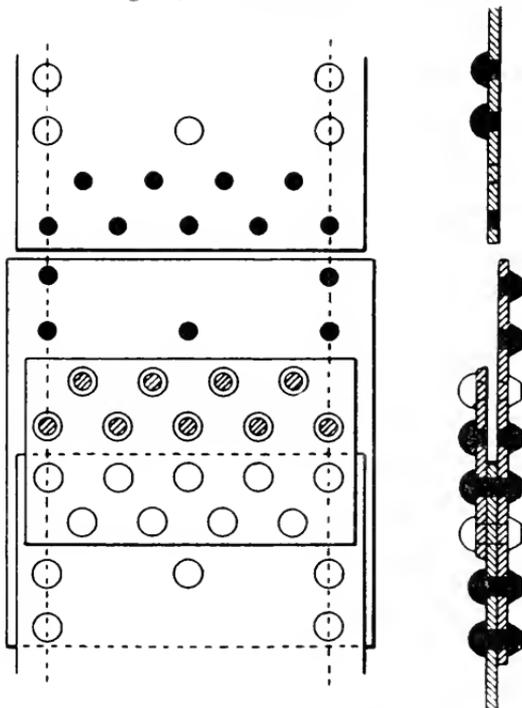
FIG. 6.—ALL THE RIVETS SHEARED.
