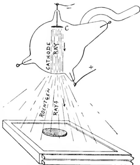
FIG. 5.—SHOWING THE RELATION OF THE ROENTGEN RAYS TO THE CATHODE RAY.
