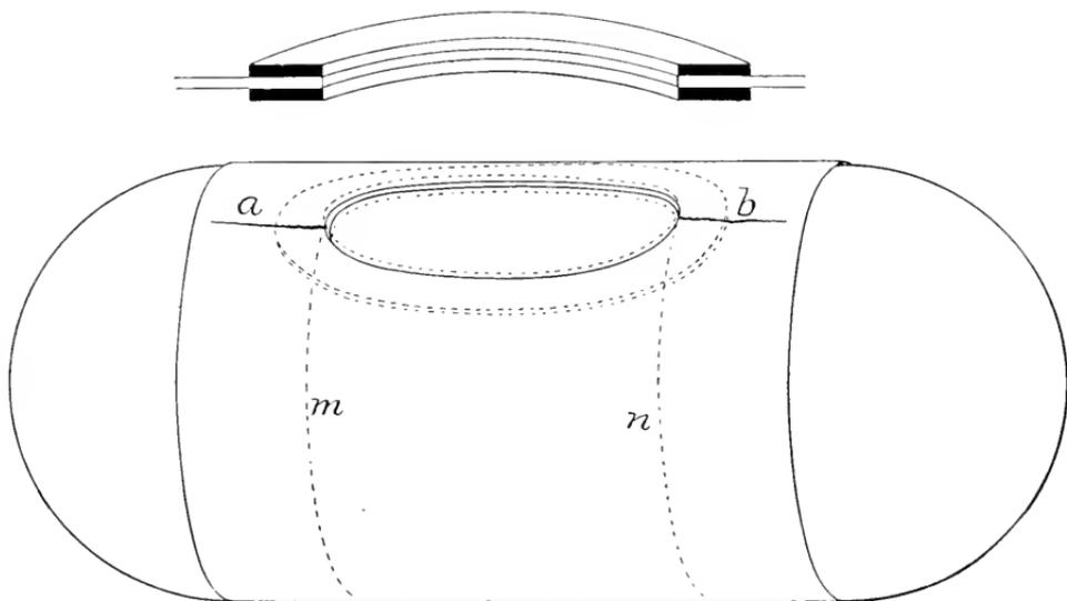
FIG. 1.—DIAGRAMATIC REPRESENTATION OF A ROTARY BOILER.
