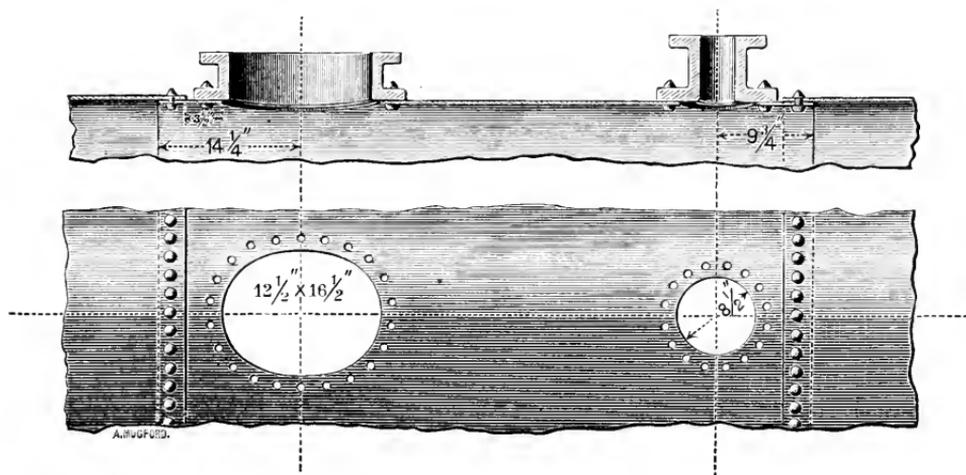
FIG. 1.— FAULTY LOCATION OF A MAN-HOLE.
