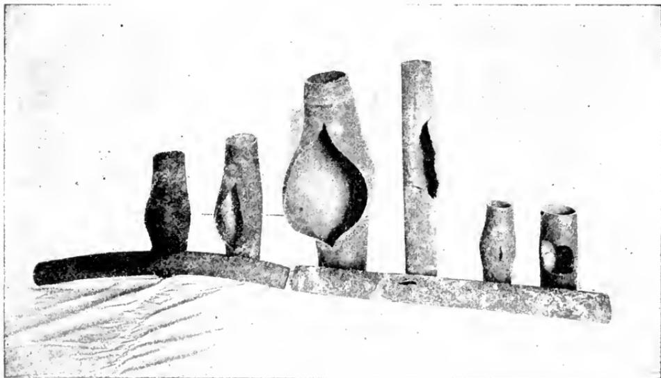
BURSTED BRASS BLOW-OFF PIPES.
