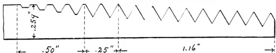
FIG. 4. — SECTION THROUGH A FIVE-INCH PIPE.
