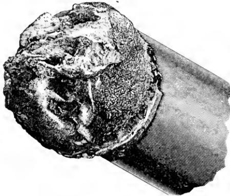
FIG. 1.—A FEED-PIPE NEARLY SEALED UP BY SCALE.
