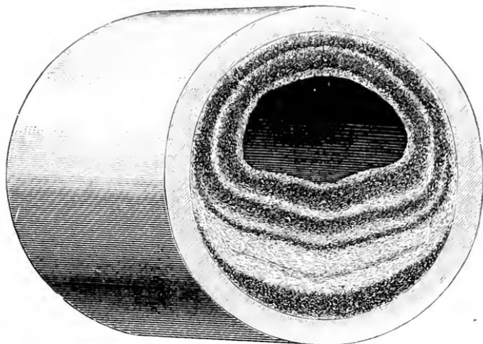
FIG. 2. — A FEED-PIPE CONTAINING A HEAVY DEPOSIT.
