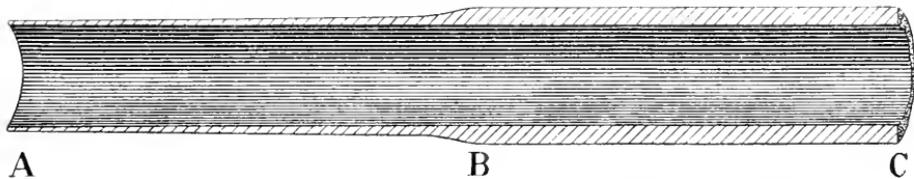
FIG. 7. — A BRASS BLOW-OFF PIPE, WASTED AWAY EXTERNALLY.
