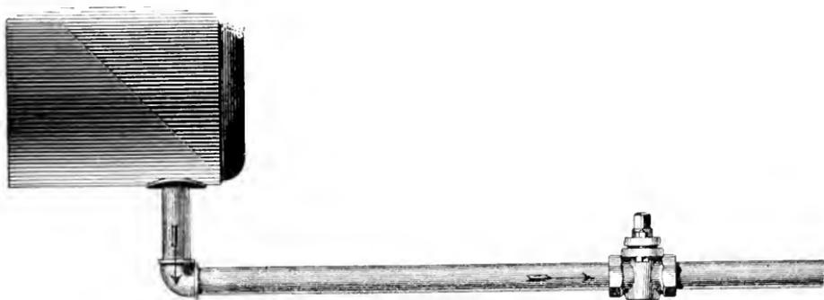
FIG. 3.—ILLUSTRATING THE "WATER RAM" IN BLOW-OFF PIPES.
