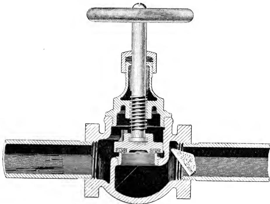
FIG. 1. — A GLOBE VALVE APPLIED TO A BLOW-OFF PIPE.
