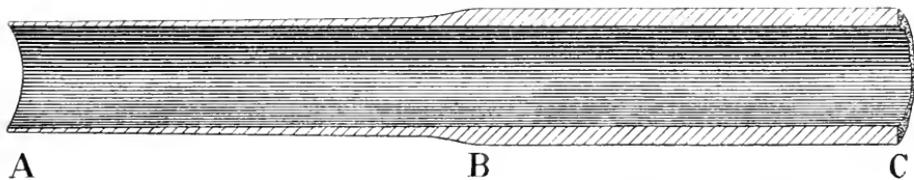
FIG. 7. — A BRASS BLOW-OFF PIPE, WASTED AWAY EXTERNALLY.
