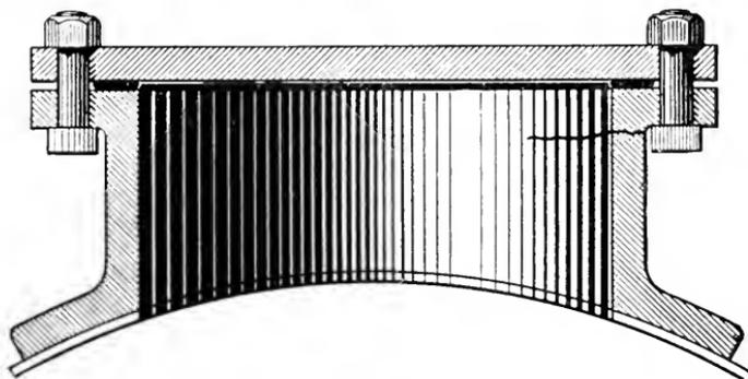
FIG. 1. — A CAST-IRON FLANGE WITHOUT BRACKETS.
