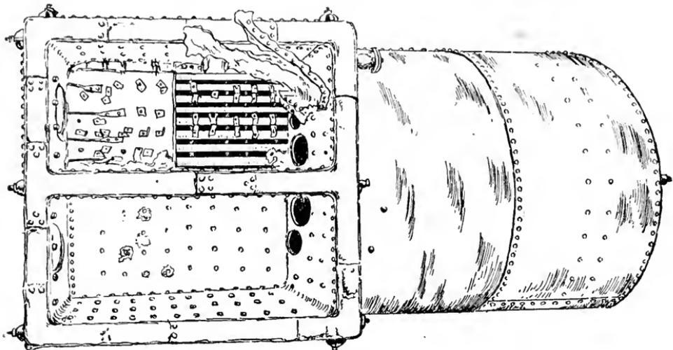
FIG. 3. — THE EXPLODED BOILER, SEEN FROM BELOW.
