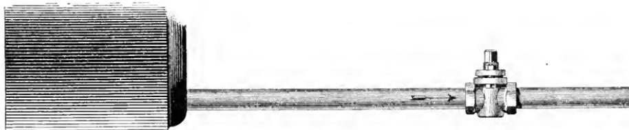
FIG. 4.—ILLUSTRATING THE "WATER RAM" IN BLOW-OFF PIPES.
