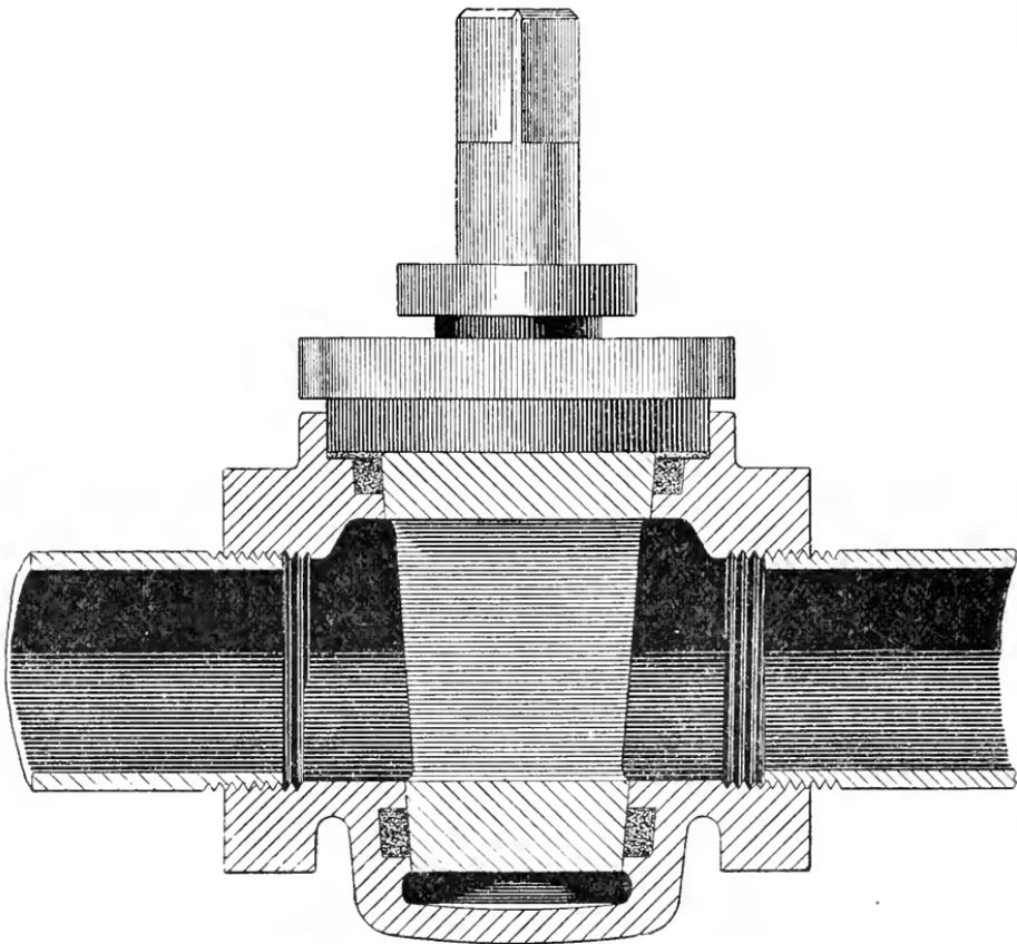
FIG. 2 — A PLUG COCK ON A BLOW-OFF PIPE.
