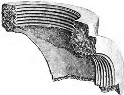
FIG. 5. — A BROKEN FITTING.
