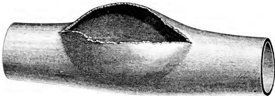
FIG. 6. — A RUPTURED BRASS BLOW-OFF PIPE.
