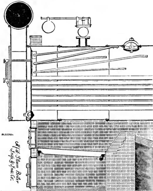
FIG. 4. — SECTIONAL VIEW OF OVERHANGING FRONT.
