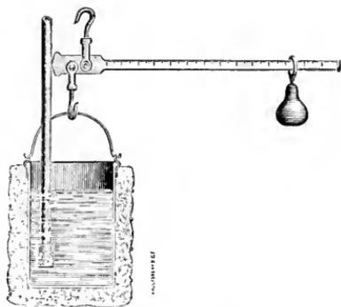
FIG. 2. — CALORIMETER.
