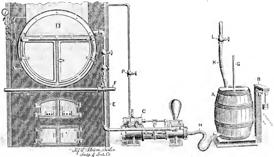
FIG. 1. — APPARATUS FOR EVAPORATIVE TEST.
