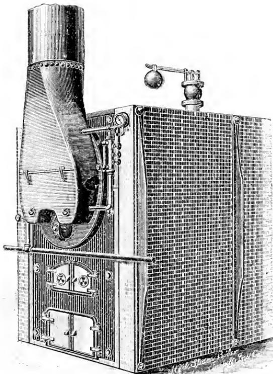
FIG. 7. — A BOILER WITH BREECHING.
