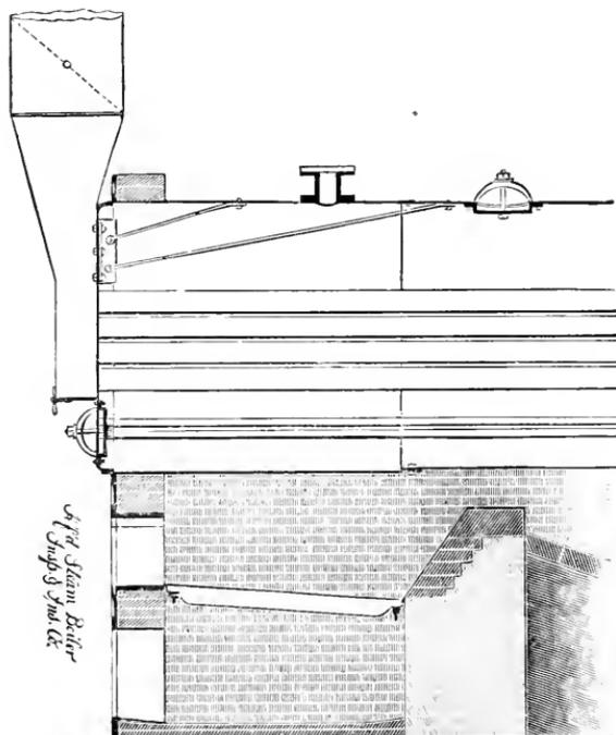
FIG. 2.—BOILER FRONT WITH BREECHING. SECTIONAL VIEW.
