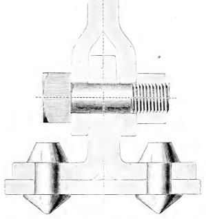
FIG. 5. - BRACE FASTENING AS IT SHOULD BE.
