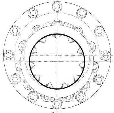
of pipe, and with especial advantage to fittings used in steam-heating systems. With the ordinary style of couplings, when the size of a steam main is reduced, it is necessary to put in a relief or drip pipe, sometimes at considerable expense and trouble, whereas if an eccentric reducing coupling were used, which would cost no more than one of the ordinary kind, the water of condensation would flow freely onward.
