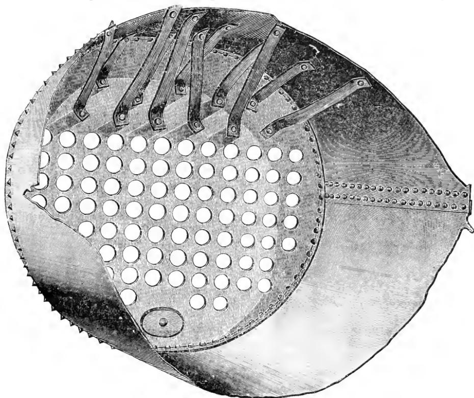
If we should construct an elastic model of an ordinary cylindrical boiler, apply pressure to it and carefully watch the effect, we should speedily observe the weakness of the heads by deflection or bulging. In some experiments made near Leeds, England, in 1876, described in "Nicholls' Practical Boiler-maker," upon an un-stayed wrought-iron boiler head, 30 inches in diameter, and  $\frac{3}{8}$  of an inch thick, the deflection carefully measured and recorded was as follows:
