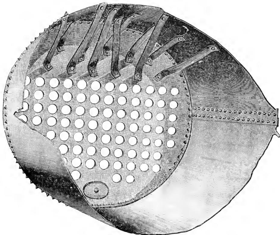
If we should construct an elastic model of an ordinary cylindrical boiler, apply pressure to it and carefully watch the effect, we should speedily observe the weakness of the heads by deflection or bulging. In some experiments made near Leeds, England, in 1876, described in "Nicholls' Practical Boiler-maker," upon an un-stayed wrought-iron boiler head, 30 inches in diameter, and  $\frac{3}{8}$  of an inch thick, the deflection carefully measured and recorded was as follows:
