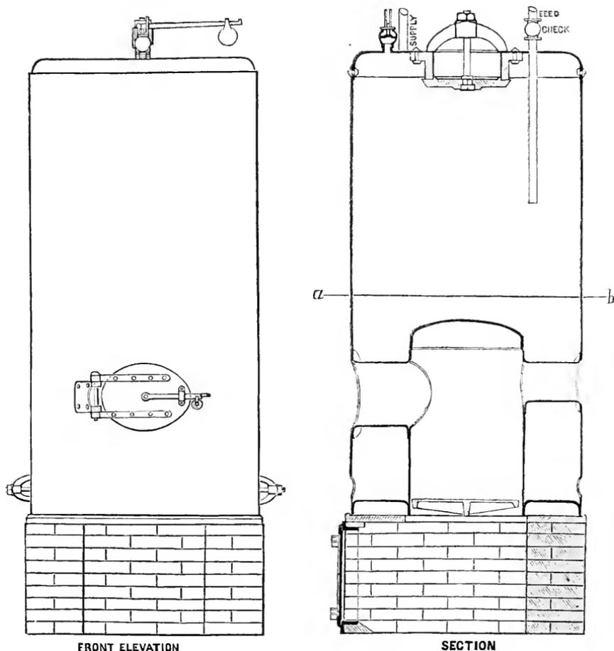
laundry, bath-rooms, and wash-bowls, in a large public institution. It is made of  $\frac{1}{4}$  inch iron, riveted up in the same manner as an ordinary vertical boiler. It sets upon a brick or cast iron base, in which is the ash pit. The grate is of the ordinary hot air furnace
