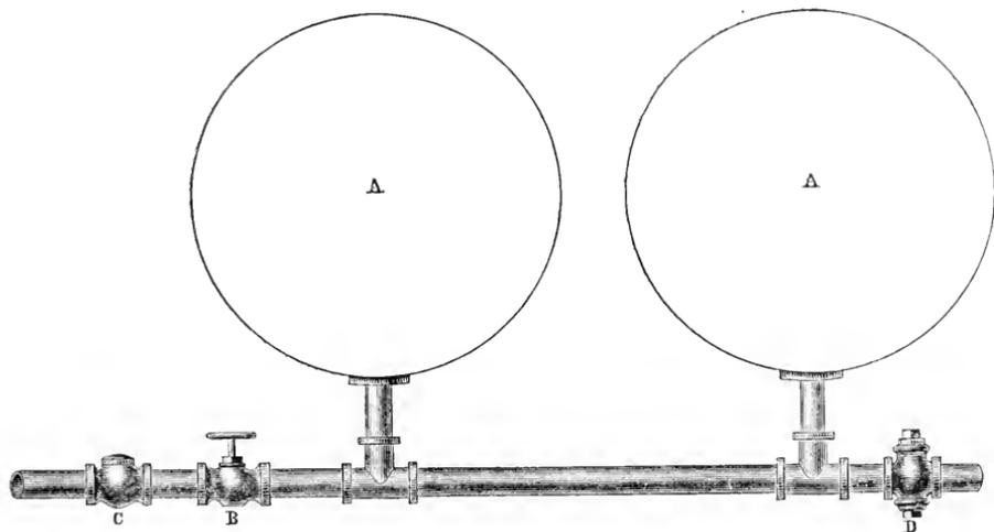
A. A.—Cross sections of two cylinder boilers,
