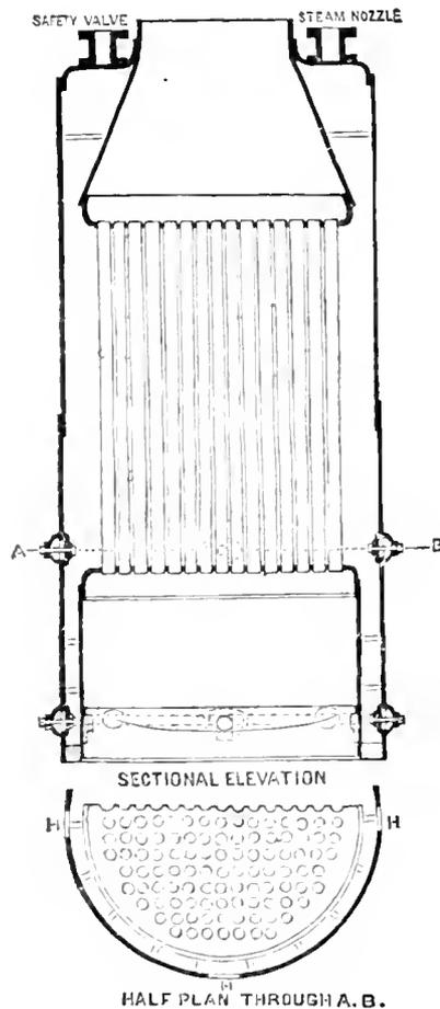
It will be seen that the upper tube-sheet is independent from the shell, but connected with a smoke-flue or uptake, which is largely below the upper head, and within the boiler. The water-line in this boiler can be maintained a little above the upper
