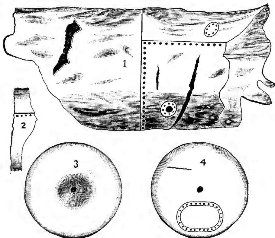
The object of the experiments was to demonstrate the truth of the theory held by Mr. Lawson that boiler explosions are caused by the opening of a valve, whereby the steam escapes, and the highly heated water remaining in the boiler thus relieved from pressure, suddenly flashes into steam, producing a concussion great enough to explode the boiler. The following table shows the results attained :
