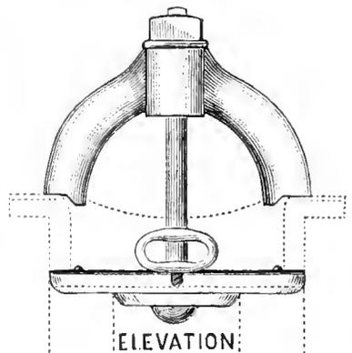
Fig. 9.— Arch and plate for inside man-hole frame.
