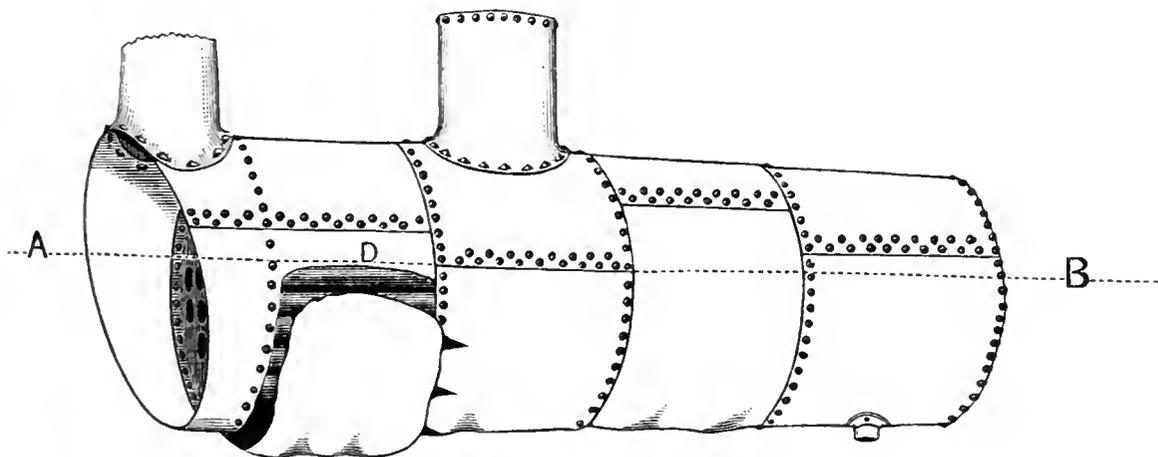
from original position over a few inches, and boilers remained inside the setting on the ground, side walls and front and back plates being thrown over on floor of mill. The cause is very evident. They have at several times had low water in boilers, and have also, contrary to our directions, blown off boilers while brick-work has been hot, thus crystalizing and hardening the iron. At the moment before the accident, they had shut down the engine preparatory to charging the re-heating furnaces.
