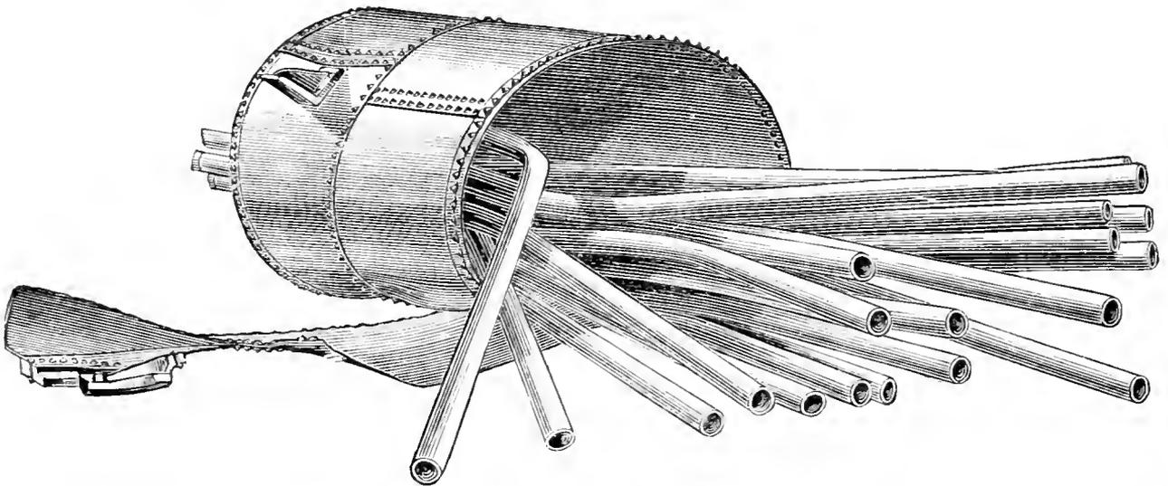
FIG. 2.—Part of No. 3 boiler, thrown 400 feet from the boiler-house.
