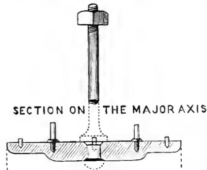
Fig. 7.— Plan for inside man-hole frame.
