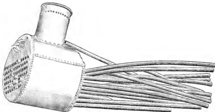
FIG. 3.—The rear end and tubes.
