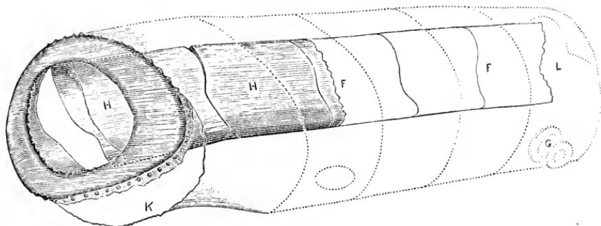
FIG. 1.—The dotted lines represent the unbroken part of the shell. The shaded portion at the left shows the foremost parts of the shell broken by the fall. The shaded portion of the flue remained in the shell, and that portion in flue outlines was blown out with the missing portion of the head at the right.
