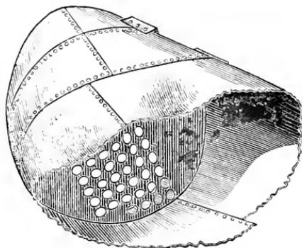
FIG. 4.—Front end of boiler.
