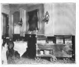
ELECTRIC WAGON, made of German silver and brass. Carries two meat platters, four vegetable compartments and one gravy. Plate warmer below and elevated service shelf above. Is about six by two feet, on heavy swivel rubber tired casters. Equipped with electric heat units, and with cord and plug to be connected to electric stations in kitchen and dining rooms.
