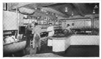
SILVER WASHING AND CLEANING DEPARTMENT (Davenport Hotel, Spokkane): Tahara machine shown open at left, with sliver in bath of shot and suds. Note the care in handling, in Particular placing the wiped sliver on mat. The Blakeside rotary sliver washing machine is located behind the solled sliver table at right. Note the sanitary enclosure of this department, all white tile wall with sanitary coved base.
