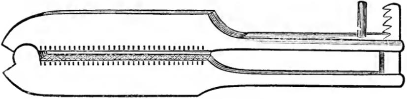
FIG. 23.—CLAMS LINED WITH VULCANIZED INDIA-RUBBER.
