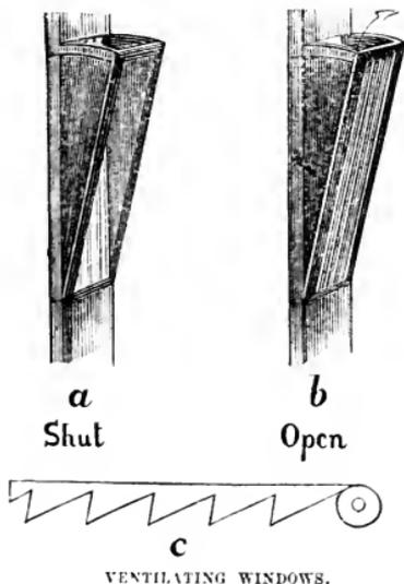
these windows may be fixed in any wall other than that at the head of the horse, but I prefer the latter as being the nearest to the nostrils where the air is wanted for the purpose of respiration.
