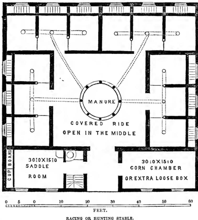
It is divided into four separate stables thirty-six feet long and eighteen wide, in which three or even four loose boxes may be separated by partitions nine feet high with open iron tops, as shown at page 172, or one or more may be divided by travises into six stalls each six feet wide. I have already alluded to the fittings for each, and therefore I need say nothing more here beyond alluding to the plan itself.\*
