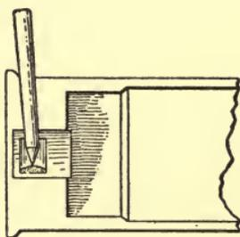
FIG. 39.—HOULLER'S PIN-FIRE IGNITION METHOD
