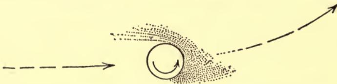
FIG. 21.—EFFECT OF UPWARD SPIN OF BULLET
