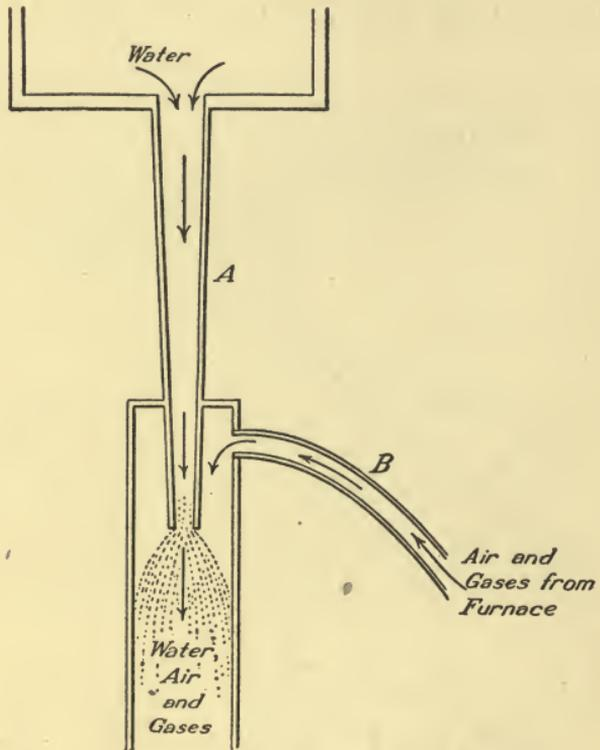
FIG. 75.—The water blast, formerly used in smelting furnaces, utilized falling water to produce air suction. In the type shown the water coming through the pipe *A* under compression sprays out of the nozzle; the falling drops, each driving air ahead of it, produce a draft through the furnace fire passing in through the pipe, *B*. Observation of the strong air currents existing at the foot of all high waterfalls probably suggested this ancient invention.
