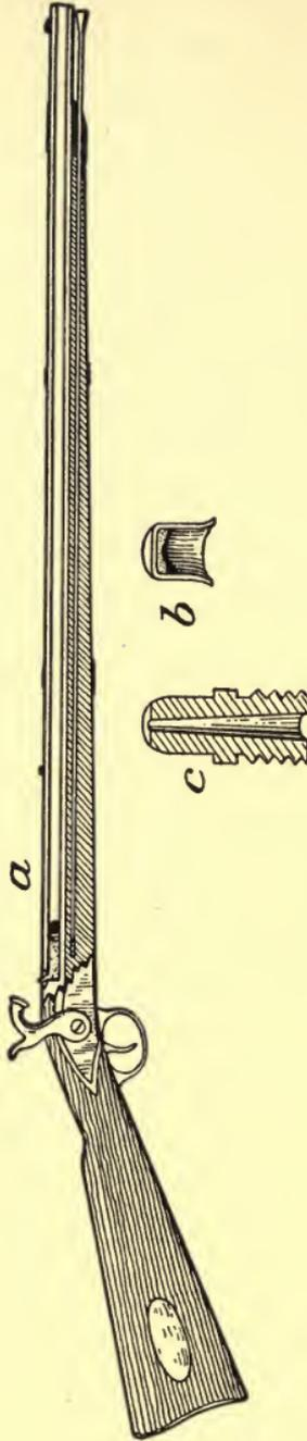
FIG. 9.—*a*, The type of musket in common use by soldiers from 1830 to 1860; *b* shows a cross-section of Shaw's percussion cap, first made of steel and then of copper; *c* is a cross-section of Shaw's nipple upon which the cup was exploded and through which the igniting flame was led into the breech in the barrel.
