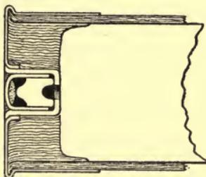
FIG. 44.—BASE OF A MODERN SHOTGUN SHELL
