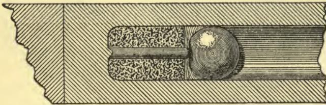
FIG. 25.—THOUVENIN CHAMBER WITH BULLET IN PLACE
