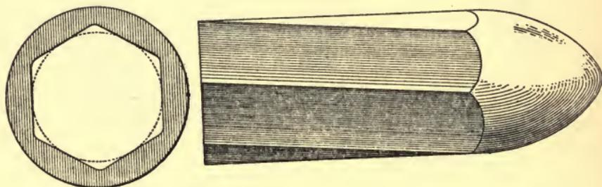
FIG. 28.—BULLET AND MUZZLE OF THE WHITWORTH RIFLE
