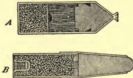
FIG. 38.—*A* and *B* are the cartridges used, respectively, in the needle gun and chassepot. The outside wrappings are of paper, the first having its primer at the base of the bullet, the other at the rear of the cartridge. A great fault with these cartridges was that the needle which exploded them quickly became corroded from contact with the burning powder, thereby often failing in operation.
