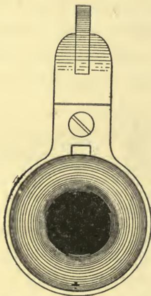
FIG. 29.—Illustrating the rifling used in our Springfield model 1906,—four lands and four grooves. The grooves are only four one-thousandths of an inch in depth, five to ten times less than those used in old-style barrels, intended for bullets of pure lead. The caliber of the bullet of course must be large enough to fill the grooves on each side; the Springfield bullet is therefore .308 caliber, while the barrel before rifling is .30 caliber.
