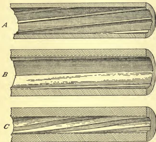
FIG. 55.—SECTIONAL VIEW OF RIFLE BARRELS
