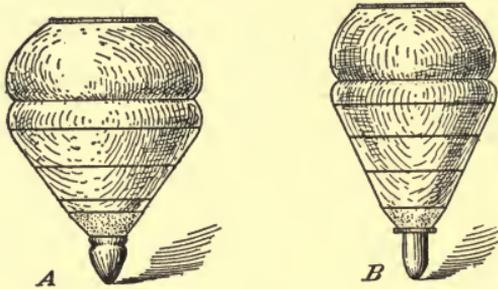
FIG. 54.—Of these two tops, *A* and *B*, the former is the thicker of the two. If both be spun at the same speed, *A* will stand up longer than *B*. Similarly the bullet with the greater diameter will remain point foremost longer than the thinner and when both are rotating at the same speed, length and material being alike.
