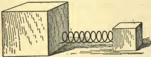
FIG. 15.—PRINCIPLES OF RECOIL
