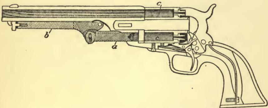
FIG. 50.—COLT'S REVOLVER, WITH JOINTED RAMROD
