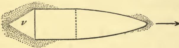
FIG. 87.—BULLET WITH FLAT END
