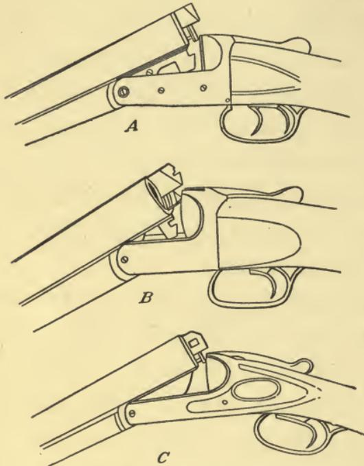
FIG. 79.—TYPES OF SHOTGUN BOLTS
