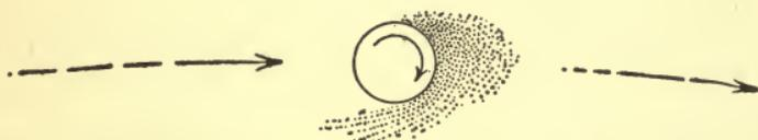
FIG. 20.—EFFECT OF DOWNWARD SPIN OF BULLET
