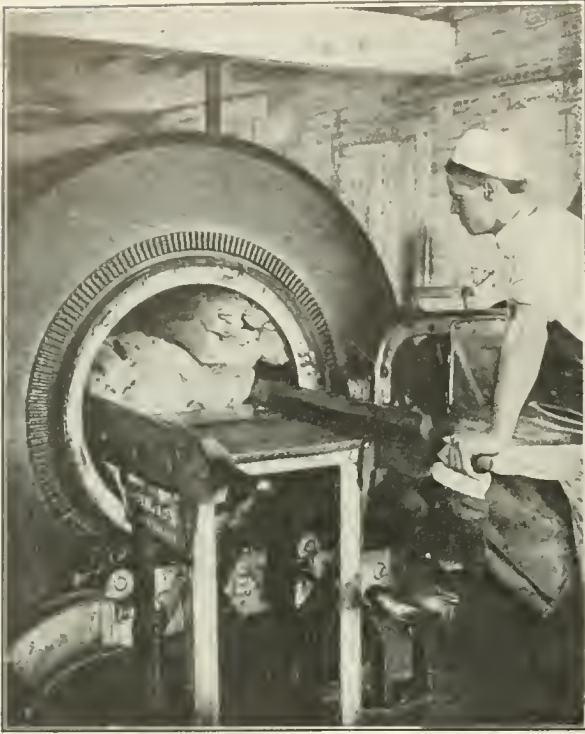
A modern churn which first converts the ripened cream into butter and then thoroughly works and salts it
