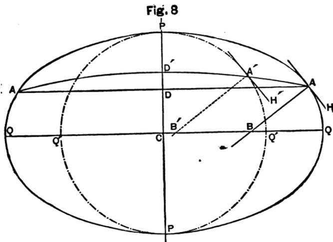
with the plane P'Q'P'Q', and becomes seen as P'Q'P'Q'. To find upon it a point A' that shall have the same latitude as A, it is only necessary to draw a tangent
