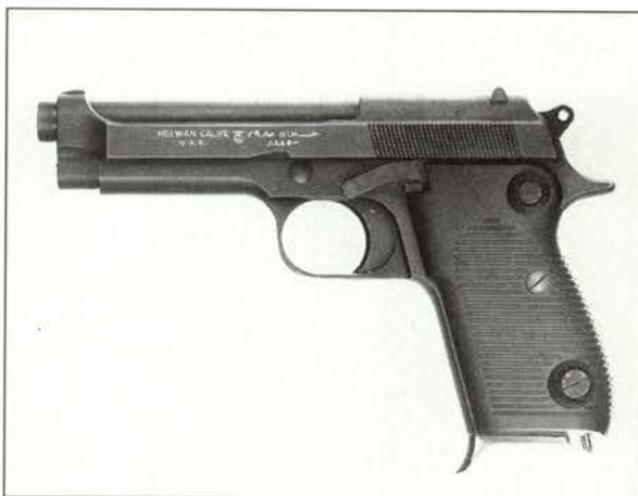
Below: Beretta Model 1951. This one was made under licence and supervision in Egypt and is known as the Helwan.
