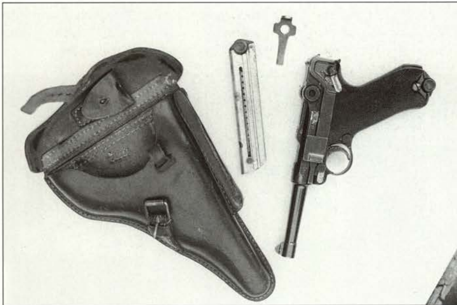
Left: P08 DWM 9mm Luger pistol, shown here with issue flap holster, spare magazine and the stripping tool, which lives in the small pouch inside the top flap. The safety catch is in the 'on' position.
