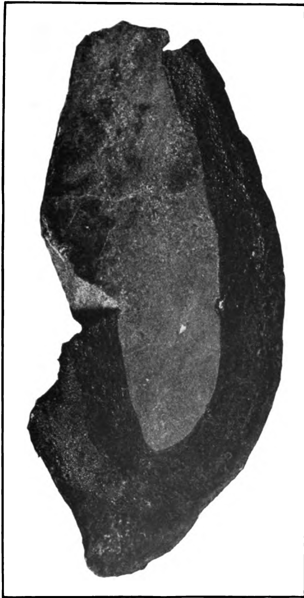
COVELLITE REPLACING ZINC SULPHIDES, FROM HORN SILVER MINE, SAN FRANCISCO REGION, UTAH.
