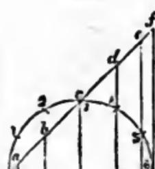
FIG. 9.—Draw a profile of half of the elbow wanted, and mark a semicircle on the line representing the diameter, divide the semicircle into six equal parts, draw perpendicular lines from each division on the circle to the angle line as on figure.
