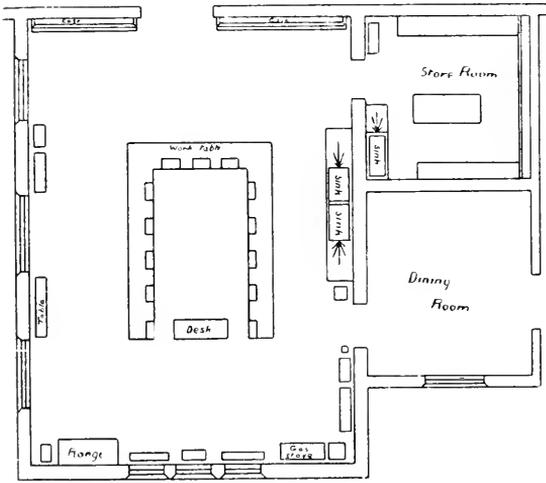
Fig. 53. Plan showing Horseshoe Arrangement of Cooking Tables.
