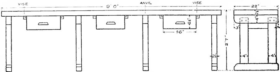
Fig 22. Metal Working Bench.
