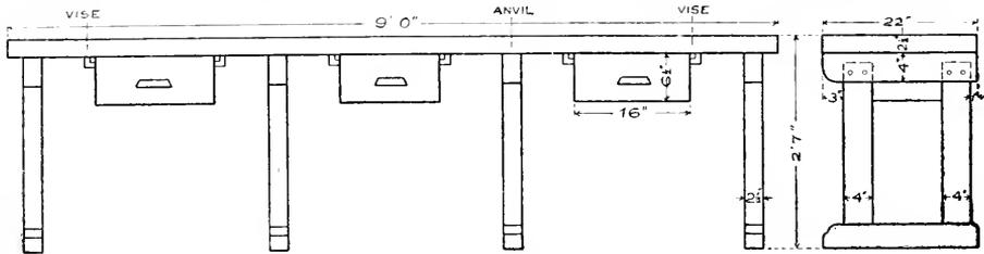
Fig 22. Metal Working Bench.
