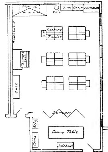
Fig. 54. Plan showing Group Arrangement of Cooking Tables.
