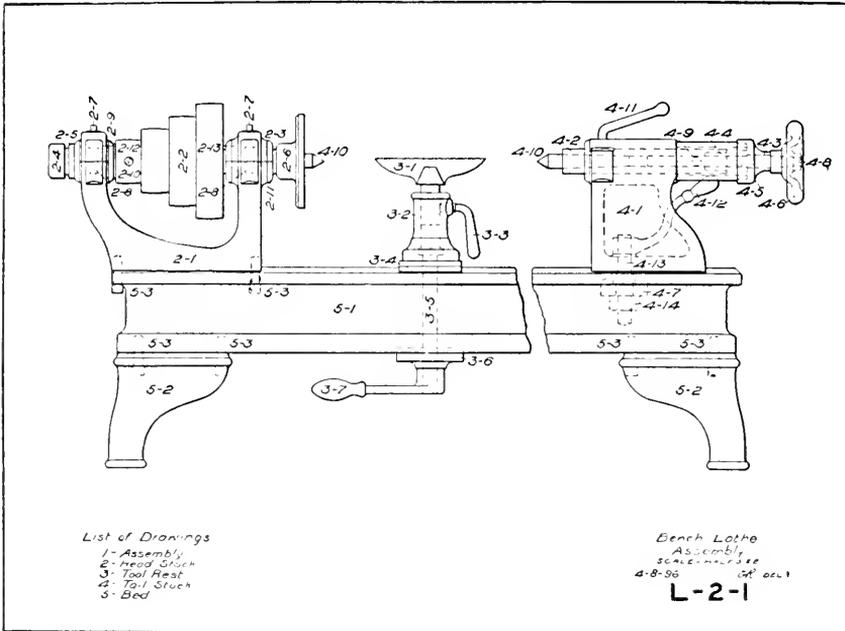
Fig. 33. Bench Lathe—Assembly.
