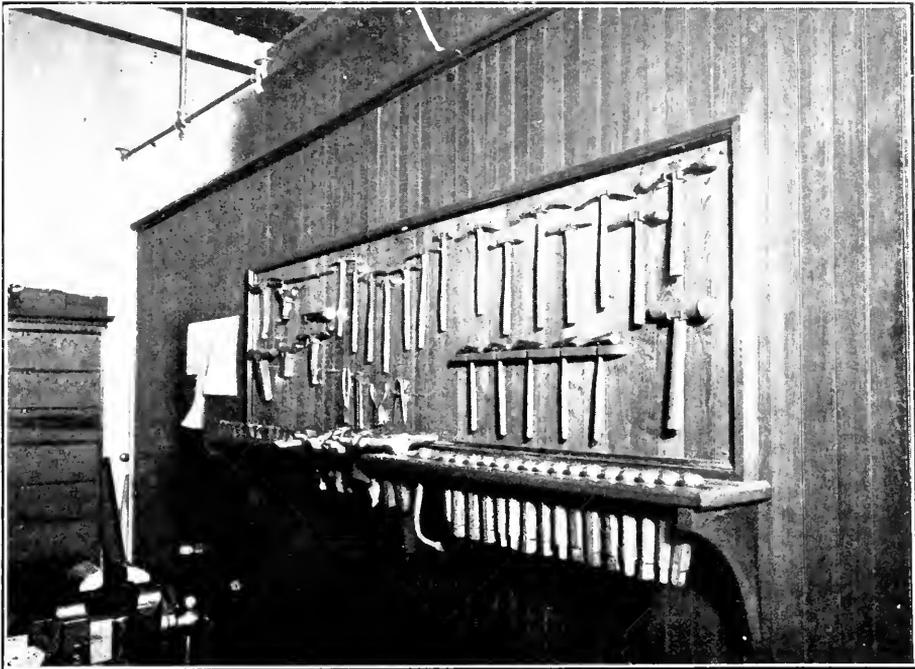
Fig. 46. Panel of Sheet Metal Working Tools.
