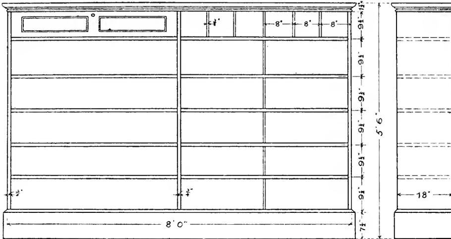
Fig. 25. Lockers for Wood Working Room.
