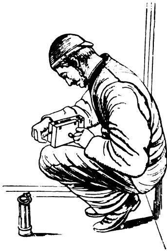
Fig. 562.—LIVEING'S INDICATOR IN USE IN THE MINE.
