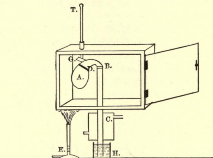
consists of a copper retort A, of about 200 c.c. capacity, detachable at D to admit of filling and subsequent cleaning. G is a small opening for admission of coal gas. (This may be dispensed with, but when used it should be freed from moisture by passing through  $\text{CaCl}_2$ .) The copper tube leading from the retort is connected at B to the glass condenser C. A copper oven, open at the bottom excepting for a covering of copper gauze, is fitted over the apparatus as shown. It contains
