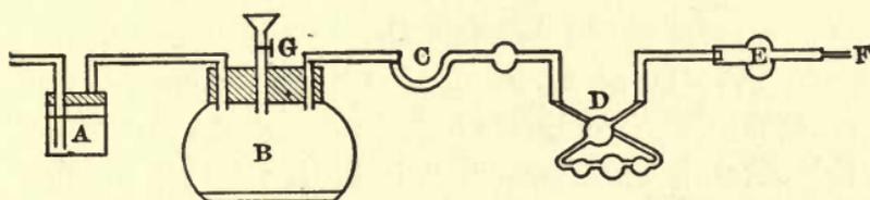
**APPARATUS.** — A is a bottle containing potash which serves to prevent any  $\text{CO}_2$  from the air entering the apparatus, and through it air is drawn into the flask B, in which the carbonates are decomposed. B contains a stoppered funnel tube G, and is connected with the calcium chloride tube C, which serves to prevent moisture from entering the potash bulbs D. E is another calcium chloride tube and is connected with the aspirator at F.
