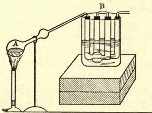
verized sample in the flask A, and pour over it concentrated  $\text{HCl}$ . At once connect A to B, in which is a solution of  $\text{KI}$ , the containing tubes being kept cool by filling the beaker about one half full of water. Now apply a burner to A and heat the solution until the sample is completely dissolved and all the evolved chlorine has been expelled and
