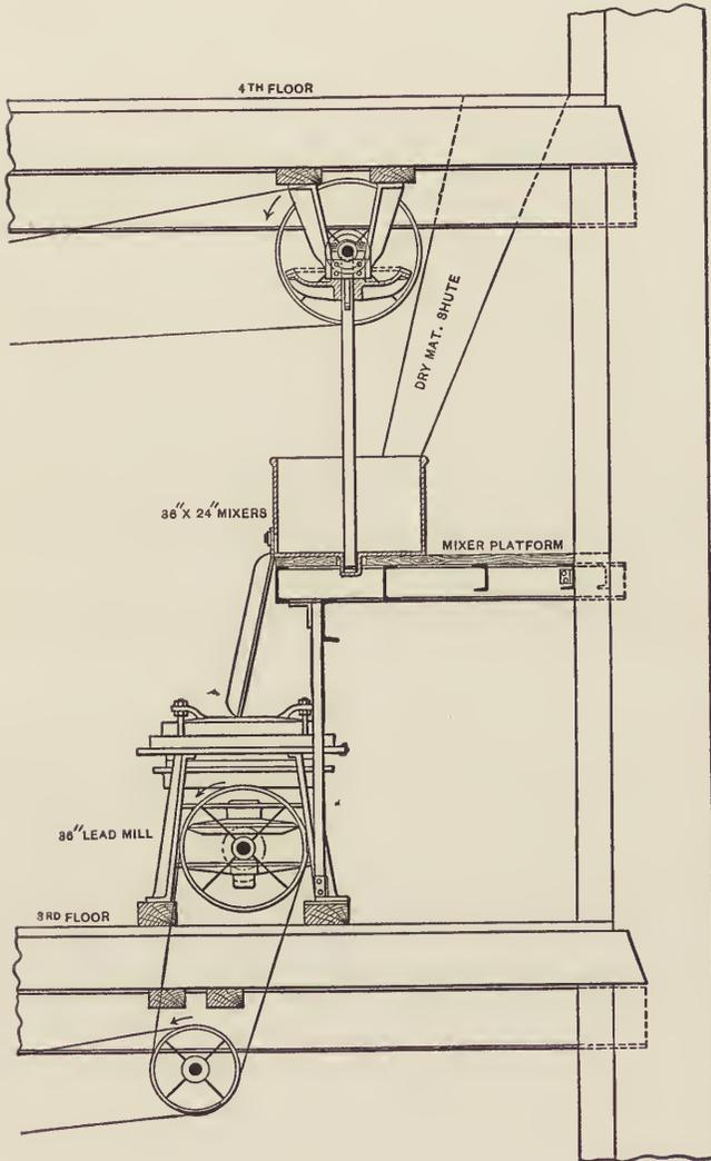
the back of this paste mill, and close to the discharge scraper, is a steel tank of generous dimensions (usually 500 gallons), into which the ground pigment is discharged. This steel tank is provided with a stirrer for mixing the ground pigment with the oil and other thinners that are added to it, in order to reduce it to a liquid form. It is then carried to the tinting tanks by a pipe-line on the same general plan as that heretofore described.
