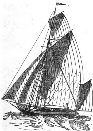
DANDY-RIGGED CUTTER, WITH JIGGER.
