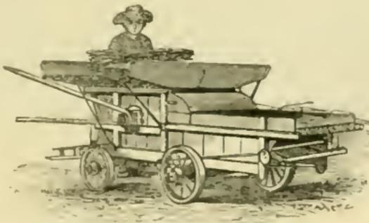
cylinder inside with an iron wheel at each end united by bars of iron; this wheel revolves by steam, causing the bars to fall upon the corn with a gliding motion, thrashing out the grain, which falls through and is received below.
