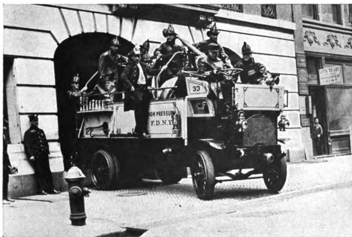
The High Pressure Wagon This is the modern Fire Engine in cities where high pressure water systems are maintained.
