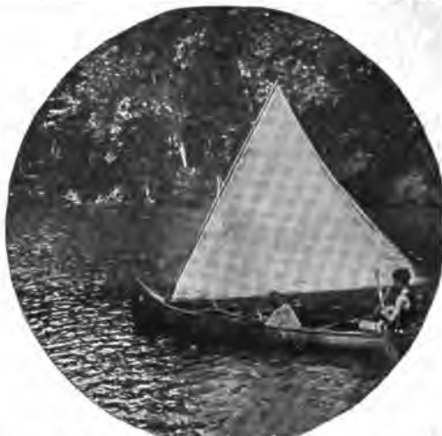
Lateen rig for open paddling canoe. This is about as much sail as this type of canoe can carry
