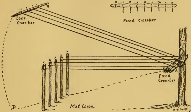
A 3-foot cross-bar *A* is fast to a small tree, and seven feet away, even stakes are driven into the ground 8 inches apart, each 3 feet out of the ground.
