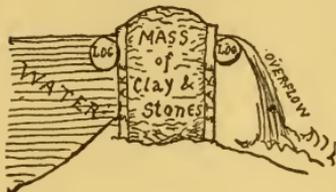
This cribbing we now filled with clay dug out of the bed of the brook above the dam. Hammering it down hard, and covering the top with flat stones.
