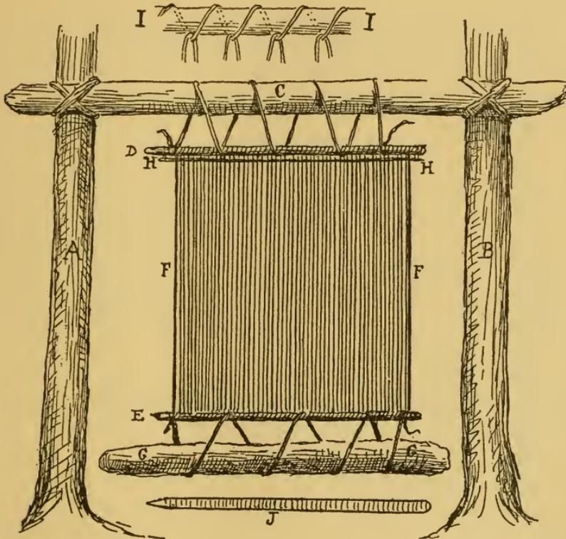
Run the batten through alternate threads again, but the reverse way of last, and this time it goes more slowly for the lack of a guide rod.\* Lay a new line of woof as
