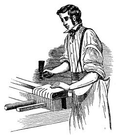
The back of the book being thus rounded, a groove is thereby formed, into which the mill-board is adjusted; the covers being fastened by the strings through the boards. The book, after
