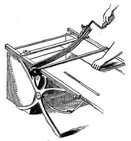
The above engraving represents the machine by which the boards are cut. These shears are so arranged that they are made to cut with perfect accuracy, according to any pattern. The preparatory process for binding in leather varies somewhat from the foregoing, which relates to books bound in muslin. The embossing machine, delineated in the following
