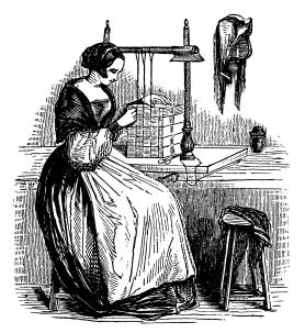
top by a cross-bar. Each successive sheet is laid flat on the bed of the sewing-press, with the back edge in contact with the strings, then opened in the middle, and fastened to the strings by passing a threaded needle backward and for-
