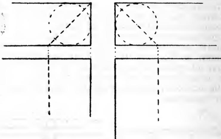
Fig. 181.—Setting out of Rule Joint.
