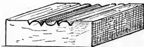
Fig. 62.—Beads with Hollow between.
