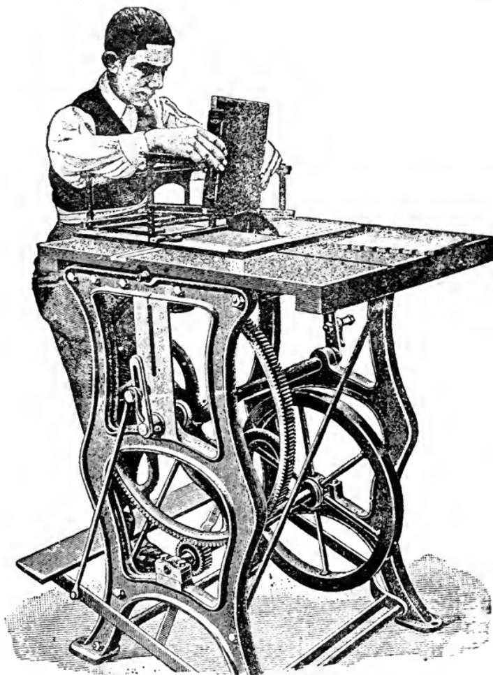
Fig. 76.—Circular Saw with Dovetailing Appliance.
