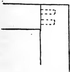
Fig. 98.—Dowel-jointed Frame.
