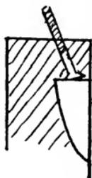
Fig. 168.—Screw through Rail.
