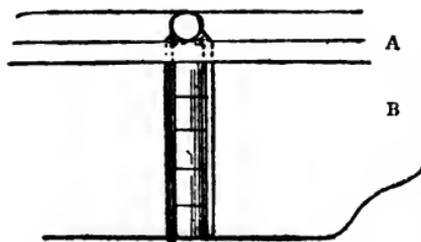
Fig. 180.—Knuckle Joint.
