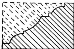
Fig. 130.—Moulding from Solid.
