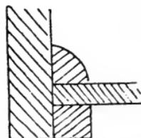
Fig. 137.—Alternative Fitting for Drawer Bottom.
