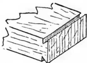
Fig. 88.—Dovetail on End.
