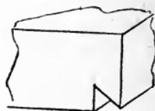
Fig. 89.—Dovetail, One End.
