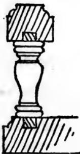
Fig. 172.—Fitting of Spindles.
