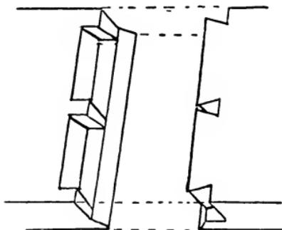
Fig. 86.—Formation of Mitre-cap Dovetails.
