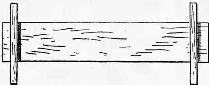
Fig. 74.—Winding Sticks on Board.
