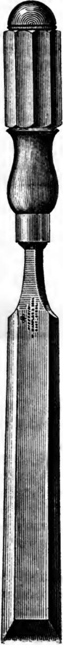
Fig. 17.—Paring Chisel.
