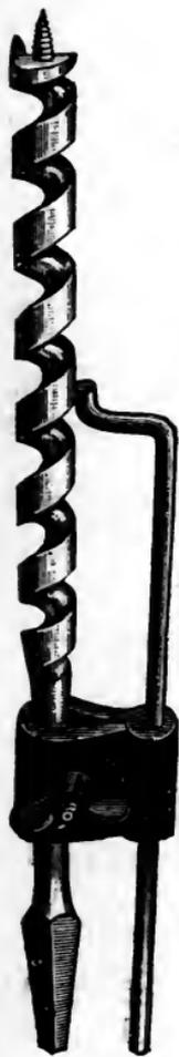
Fig. 27.—Twist Bit and Gauge.
