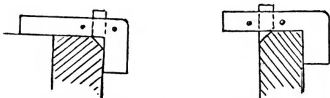
Figs. 65 and 66.—Scraper for Chamfering.
