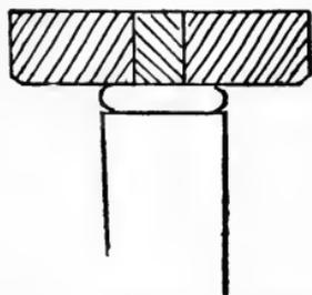
Fig. 170.—Fitting of Legs to Rails.
