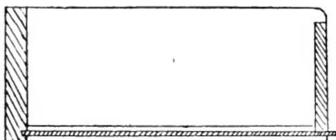
Fig. 136.—Drawer Side with Bottom, &c.
