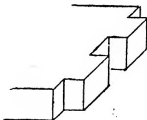
Fig. 96.—Tenons on End of Shelf, &c.
