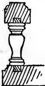
Fig. 172.—Fitting of Spindles.
