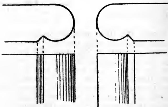
Fig. 182.—Shaping of Wood for Rule Joint.
