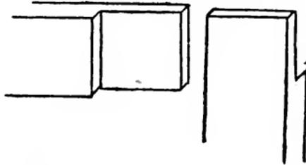
Fig. 99.—Halved Corner Joint.
