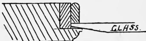
Fig. 158.—Transparent Bevelled Glass fitted.
