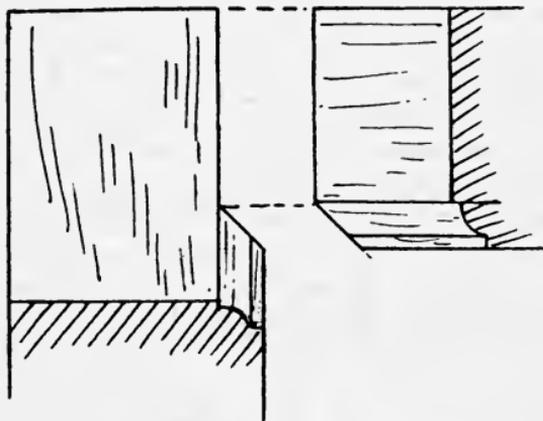
Fig. 147.—Mitred Mouldings Worked on Frame.
