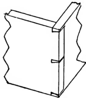
Fig. 84.—Ditto, with Badly-formed Pins.
