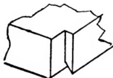
Fig. 90.—Dovetail Stopped Back from Front.
