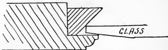
Fig. 157.—Bevelled Glass blocked.
