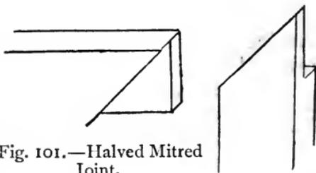
Fig. 101.—Halved Mitred Joint.
