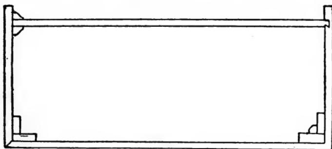
Fig. 149a.—Plinth or Cornice showing Fastenings.
