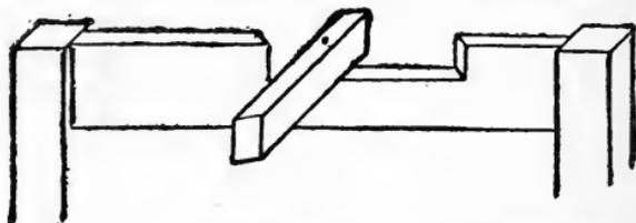
Fig. 184.—Pinned Rail for supporting Flap.
