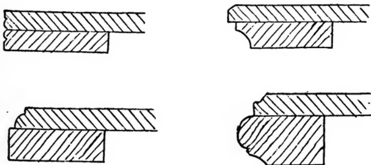
Figs. 102 to 105. — Sections of Lined-up Tops.
