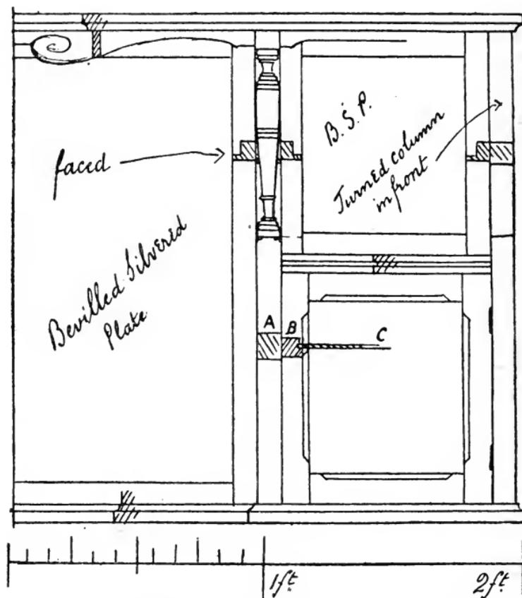
Fig. 162.—Working Drawing and Scale of Overmantel.
