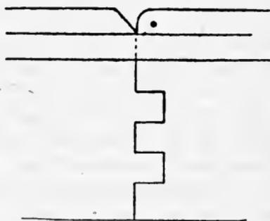
Fig. 183.—Finger Joint for Brackets.
