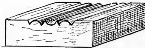
Fig. 62.—Beads with Hollow between.
