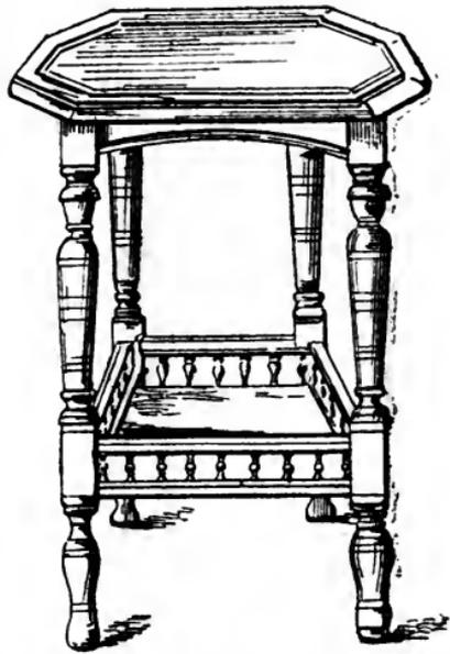
Fig. 171.—Table with Spindled Rails.
