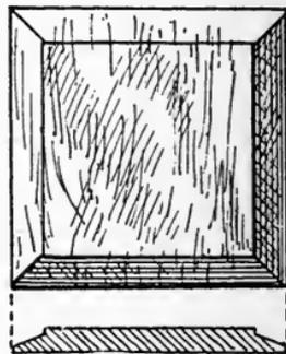
Fig. 109.—Panel with Sunk Bevelled Edges.
