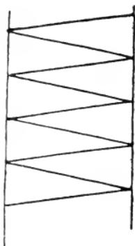
Fig. 166.—Diagram showing course of Veneering Hammer.
