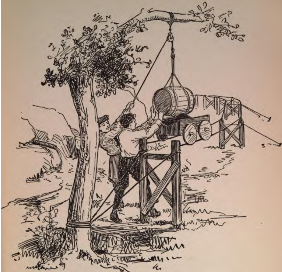
FIG. 103.—Using the wire railway to haul water from the spring to camp
