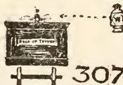
ENGINE MOVING BACKWARD BY NIGHT WITHOUT CARS OR AT THE FRONT OF A TRAIN PULLING CARS.
