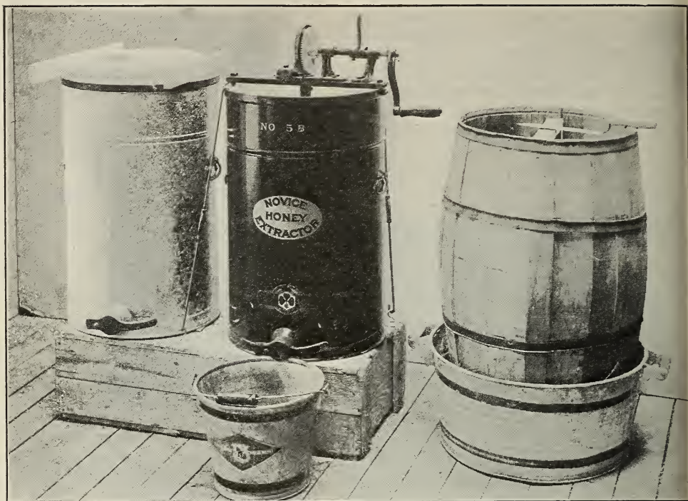
This illustration shows at the left the strainer resting by two cleats on the top of the can. The extractor is shown in center, and uncapping barrel at right.
