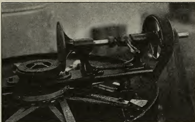
The cam lever in a horizontal position, the extractor at rest.
