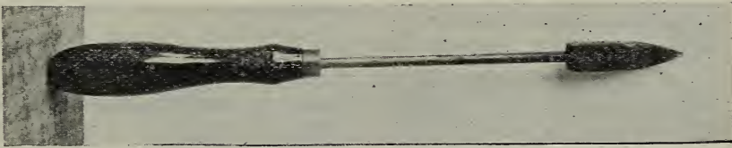
A. C. Miller's soldering iron with the point grooved so that it may be used for imbedding wires.
