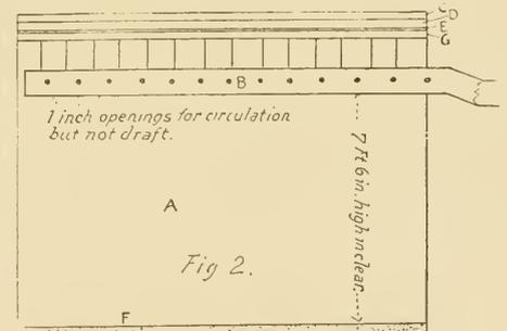
Perpendicular elevation of bee-cellar, showing the square-box ventilating-line with its one-inch holes as shown in diagram 3.
