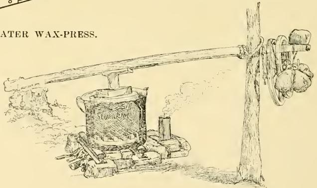
FIG. 6.—USE OF THE LEVER IN PRESSING WAX.
