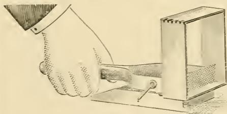
The idea is, to rub the edge of the wax into the wood of the section. The motion of the machine spreads the wax down, and mashes it into the wood, as it were. It is a very simple machine, and is used quite
