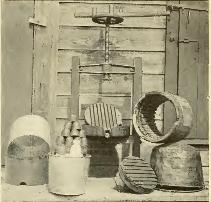
Fig. 18.—A lard-press modified for pressing wax.
