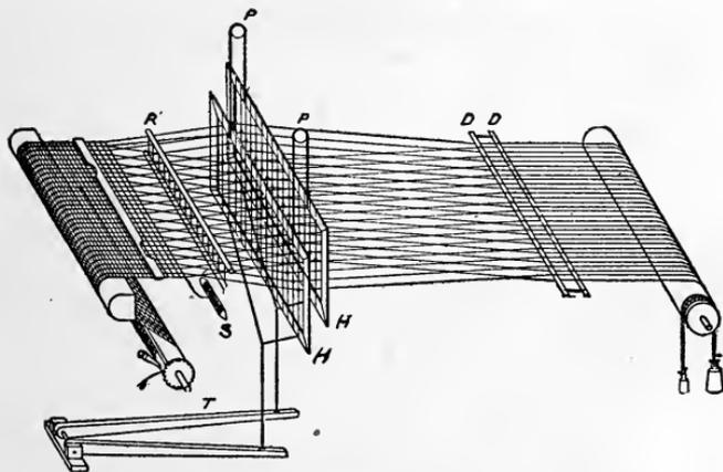
DIAGRAM OF THE WORKING PARTS OF A LOOM.
